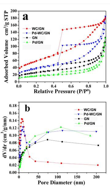
**Fig. S6** (a) Nitrogen-sorption isotherms and (b) the corresponding pore-size distribution curves of different samples.
