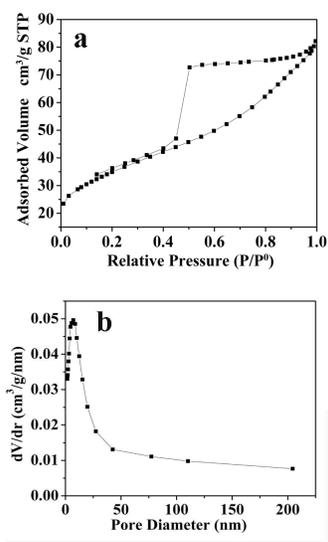
**Fig. S5** Nitrogen adsorption/desorption isotherms of  $\text{WO}_3\text{-nH}_2\text{O/GN}$  sample. (The  $S_{\text{BET}}$  of  $\text{WO}_3\text{-nH}_2\text{O/GN}$  is  $123.8 \text{ m}^2/\text{g}$ ).
