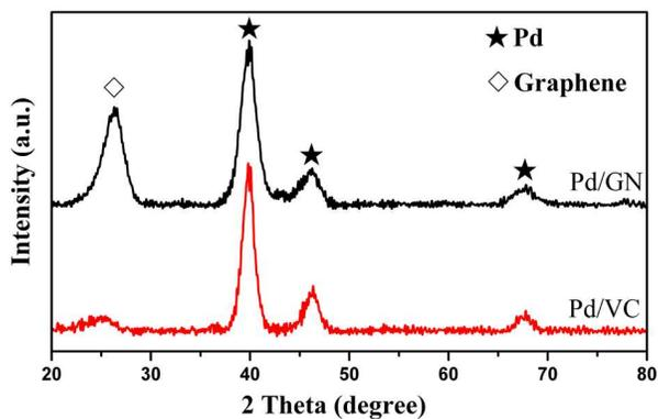
**Fig. S2** XRD patterns of Pd/GN and Pd/VC.
