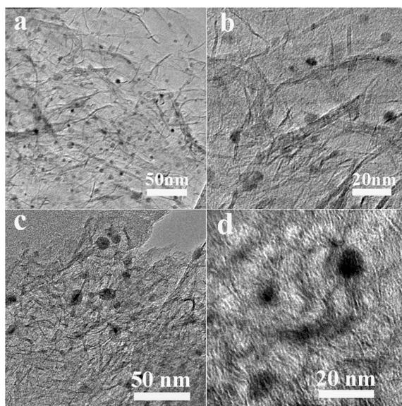
**Fig. S4** Low and high magnification TEM images of (a, b) the  $\text{WO}_3\text{-nH}_2\text{O}/\text{GN}$  sample (before thermal treating) and (c, d) the  $\text{WC}/\text{GN}$  sample (after thermal treating).
