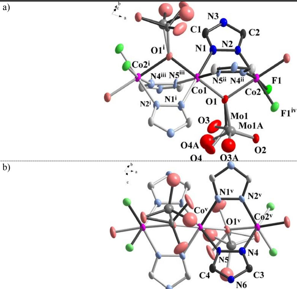
**Figure S4.** Illustration of the centrosymmetrical trinuclear fragments in the crystal structure **2**. (i) -x+1, -y+1, -z+1; (ii) x, y-1, z+1; (iii) -x+1, -y+2, -z; (iv) -x+2, -y+1, -z+1; (v) x, y+1, z-1.
