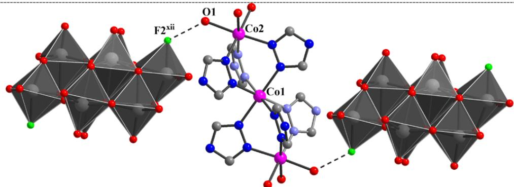
**Figure S8.** The O-H...F hydrogen-bonding interactions between coordinating water and  $[\text{Mo}_8\text{O}_{26}\text{F}_2]^{6-}$ -anions ( $\text{O}1\text{-H}...\text{F}2 = 2.843(4)$  Å) in the crystal structure of **3**; symmetry code: (xii)  $x+1, y, z$ ;
