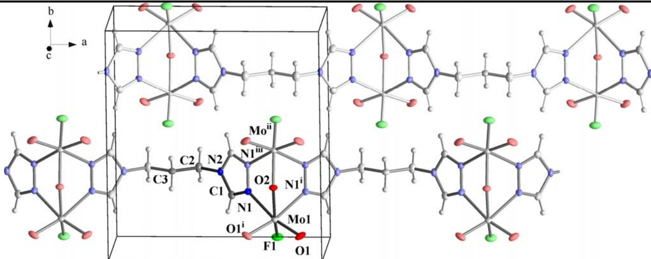
**Figure S1.** Crystal structure and labeling scheme for  $[Mo_2F_2O_5(tr_2pr)]$ , (1). Ellipsoids are shown at the 50% probability level.
