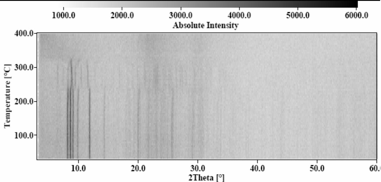
**Figure S21.** The Guinier–Simon diagram for complex **3** ( $2\theta = 5\text{--}60^\circ$ ) reveals a framework stability up to  $240^\circ\text{C}$ .
