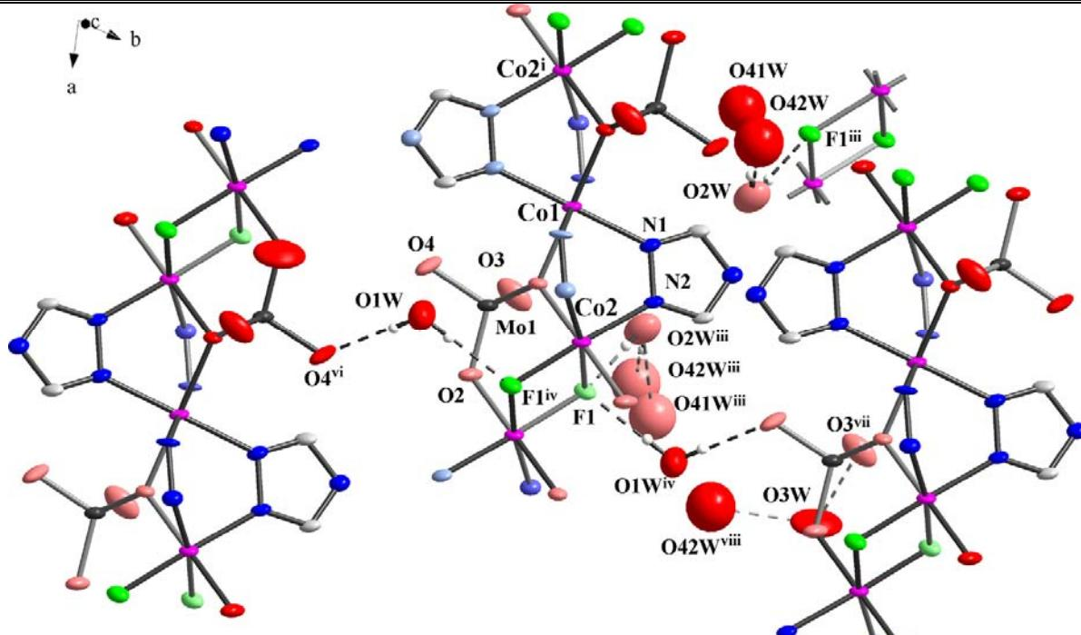
**Figure S5.** The H-bonding patterns showing the interconnections between the neighboring  $[Co_3(tr)_4(MoO_4)_2F_2]_n$  chains; symmetry codes: (i)  $-x+1, -y+1, -z+1$ ; (ii)  $x, y-1, z+1$ ; (iii)  $-x+1, -y+2, -z$ ; (iv)  $-x+2, -y+1, -z+1$ ; (v)  $x, y+1, z-1$ ; (vi)  $-x+2, -y, -z+1$ ; (vii)  $x, 1+y, z$ ; (viii)  $1+x, y, z..$
