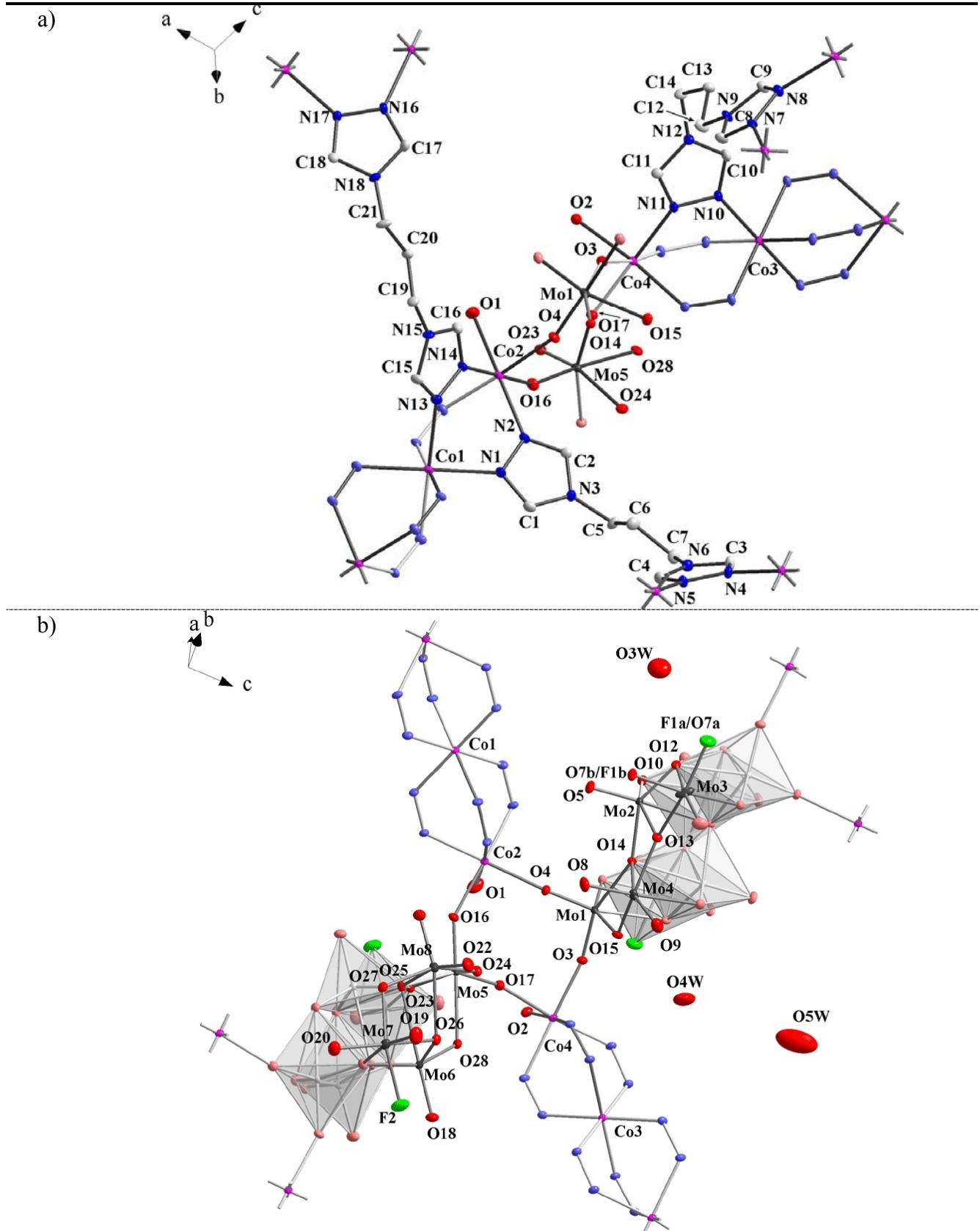
**Figure S7.** Crystal structure and labeling scheme for  $[\text{Co}_3(\text{H}_2\text{O})_2(\text{tr}_2\text{pr})_3(\text{Mo}_8\text{O}_{26}\text{F}_2)] \cdot 3\text{H}_2\text{O}$  (**3**). Ellipsoids are shown at the 50% probability level.
