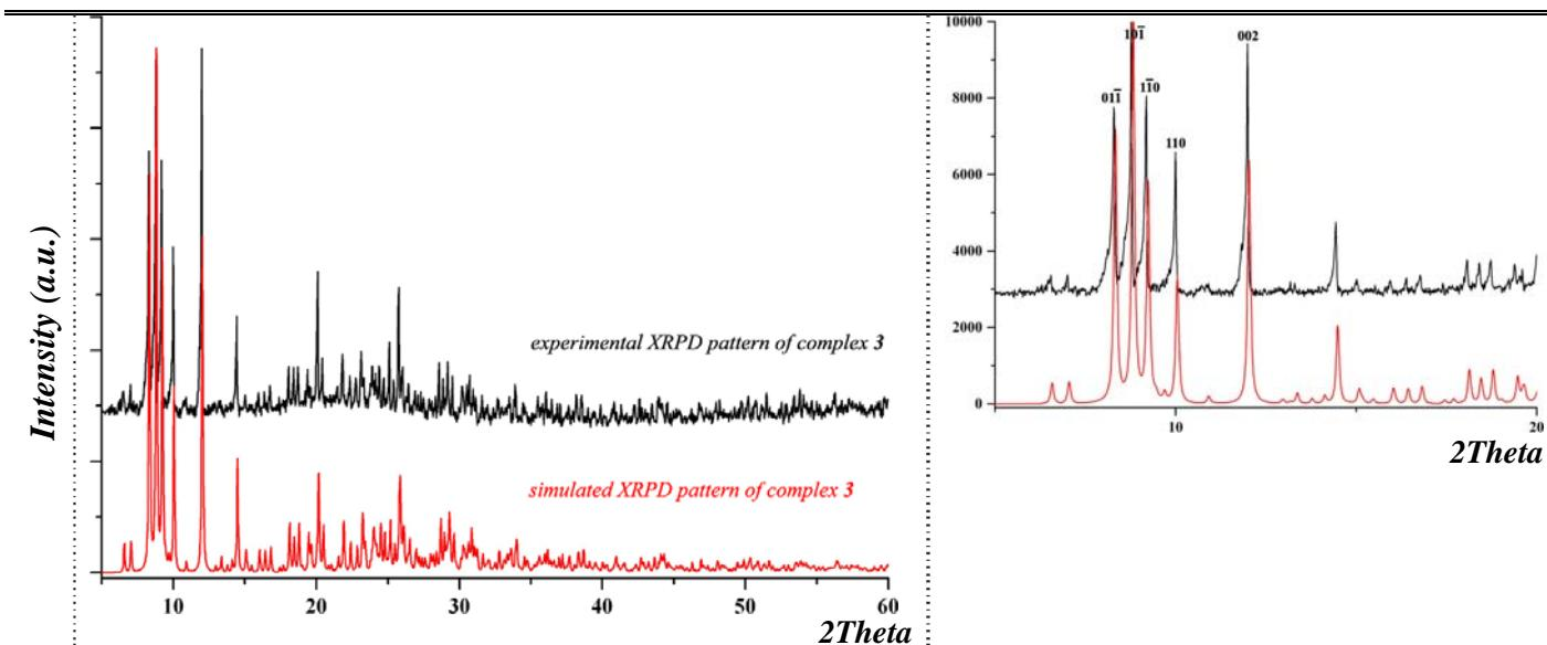
**Figure S20.** The bulk-phase purity of compound 3 was confirmed by comparing the XRPD patterns with the simulated one.
