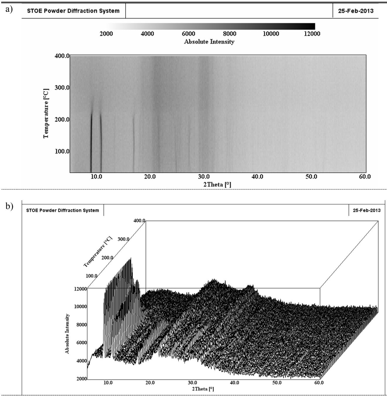
**Figure S18.** a), b). The 2D and 3D Guinier-Simon diagrams of the TD-XRPD measurements of compound 2.
