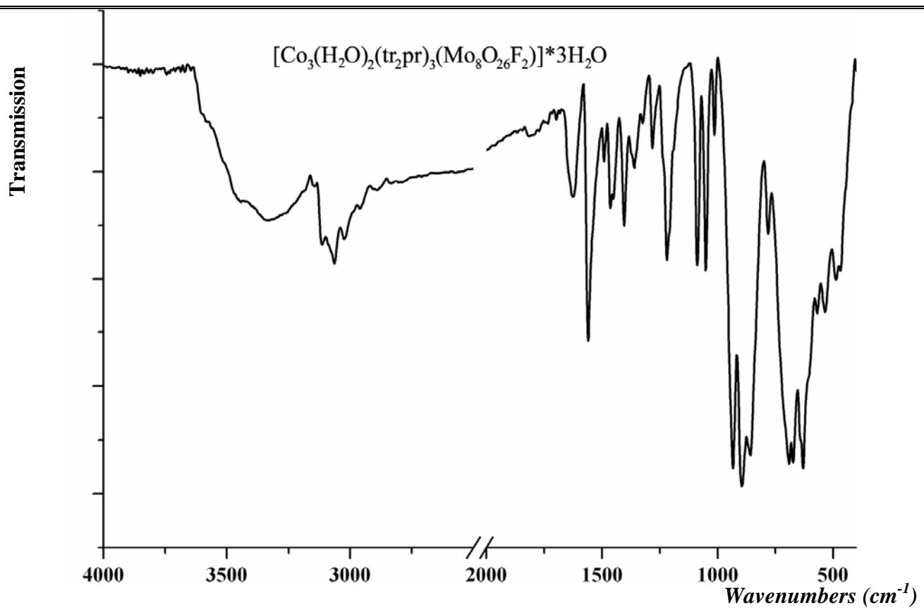
**Figure S15.** IR spectrum of compound 3.
