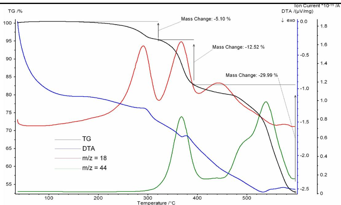
**Figure S22.** DTA and TGA data showing a weight loss (5.1 %) in the range  $165^\circ\text{C} \text{--} 310^\circ\text{C}$ , consistent with the removal of five water molecules for  $[\text{Co}_3(\text{H}_2\text{O})_2(\text{tr}_2\text{pr})_3(\text{Mo}_8\text{O}_{26}\text{F}_2)] \cdot 3\text{H}_2\text{O}$  (**3**).
