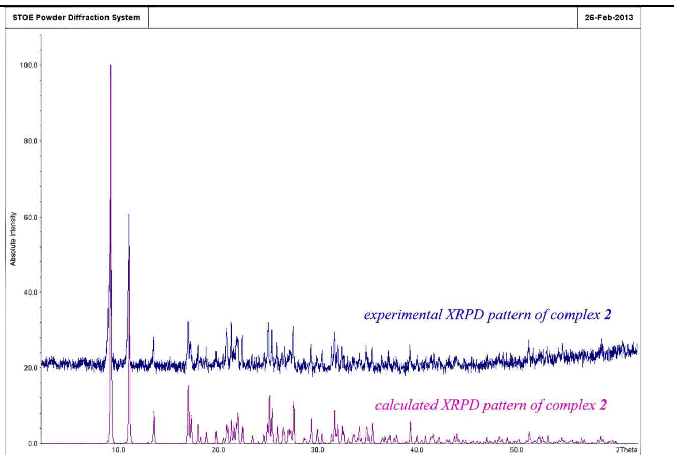
**Figure S17.** The bulk-phase purity of complex 2 was confirmed by comparing its experimental and simulated XRPD patterns.
