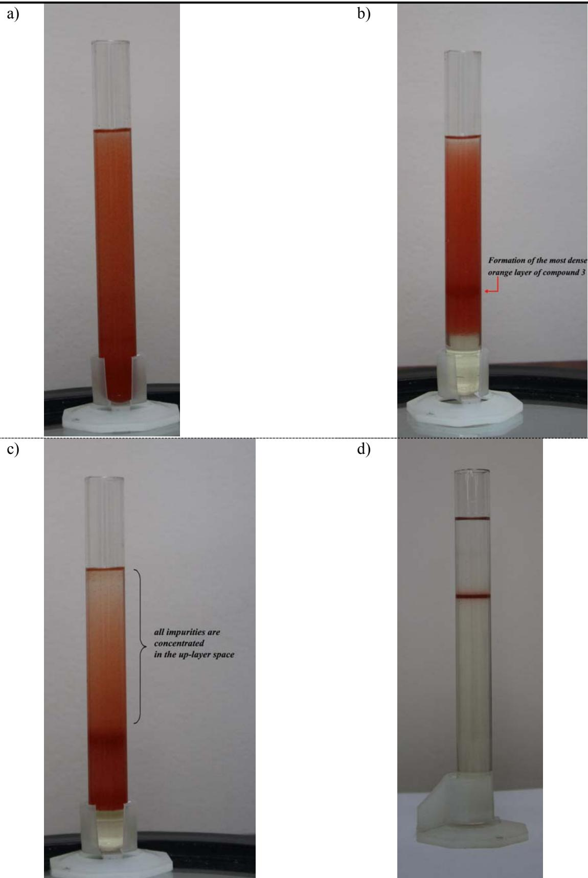
**Figure S13.** Photographs of a step-wise separation process of compound **3** utilizing a flotation method in a  $\text{CHBr}_3/\text{CHCl}_3$  solution: a) the crystalline mixture was immersed in  $\text{CHBr}_3/\text{CHCl}_3$ ; b) the bottom layer contains the most dense compound, i.g., complex **3**; c) the impurities, concentrated in the up-layer space, were removed using a Pasteur pipette. The purification steps (1-3) were repeated over and over again to receive pure phase **3**; d).
