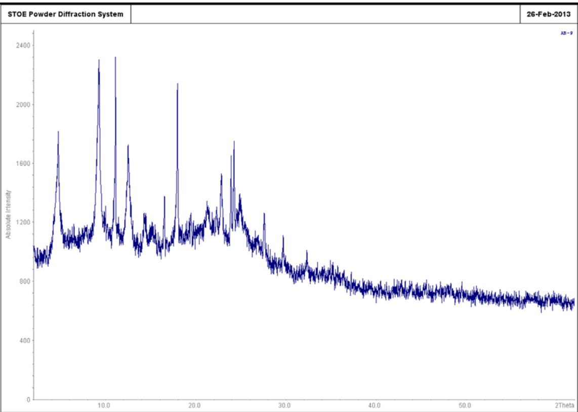
**Figure S16.** The powder XRD patterns of the unknown phase isolated from hydrothermal reaction of  $\text{Co}(\text{OAc})_2 \cdot 4\text{H}_2\text{O}$  (24.9 mg, 0.1 mmol),  $tr_{2pr}$  (17.8 mg, 0.1 mmol),  $\text{MoO}_3$  (28.8 mg, 0.2 mmol) and 100  $\mu\text{L}$  22% HF (1.18 mmol) in 5 mL of  $\text{H}_2\text{O}$ .
