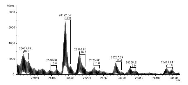
**Figure S6**. Section of the deconvolved MS spectrum of PSA-1 from an LC-ESI-MS run in the intact protein mode. Pairs of peaks are annotated which arise from protein oxidation and/or glycoforms of PSA.
