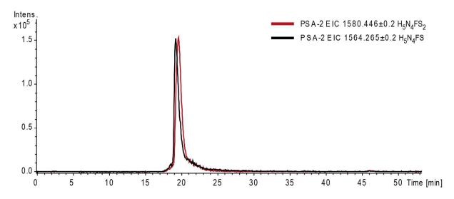
**Figure S3**. EICs of the chromatographic profiles of intact PSA glycoforms on a C8-column in a 60 min LC run. The PSA glycoform at *m*/*z* 1564.32 (complex type glycan, composition  $H_5N_4FS$ ) elutes at 19.2 min and the glycoforms at *m*/*z* 1553.92 (complex type glycan, composition  $H_5N_4FS_2$ ) at 19.6 min.
