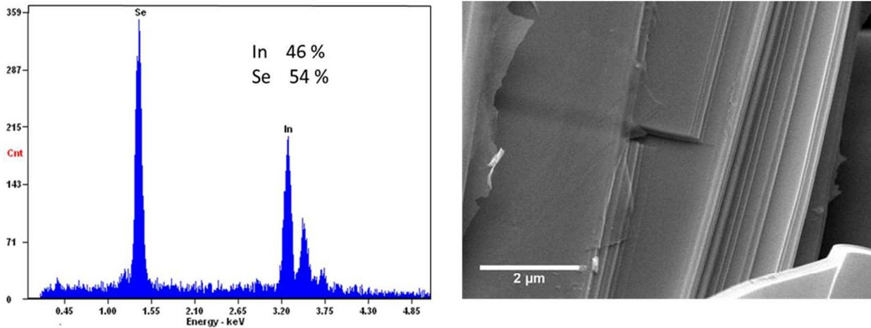
**Figure S1.** EDX spectra (left) and SEM image (right) of InSe crystal synthesized by non-stoichiometric melt method. EDX shows an elemental ratio of 1 :1 between In and Se. SEM image shows an obvious layered structure.
