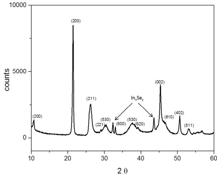
**Figure S2.** XRD spectrum of crystal synthesized by non-stoichiometric melt
