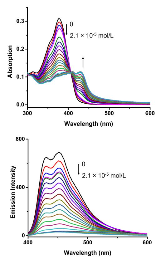
Figure S3. Absorption and fluorescent spectra of DPI-BP ( $5 \times 10^{-6}$  mol/L CHCl<sub>3</sub> solution, 3.0 mL) upon
