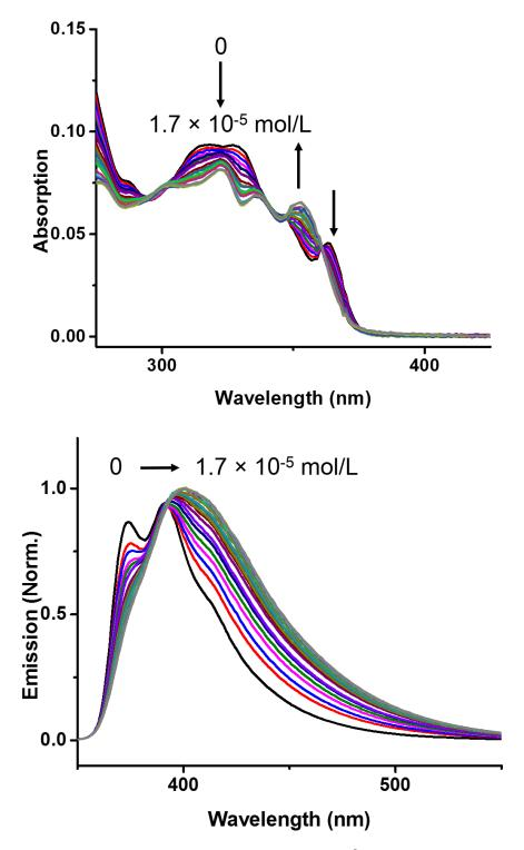
**Figure S7.** Absorption and fluorescence spectra of PI-Ph ( $5 \times 10^{-6}$  mol/L CHCl<sub>3</sub> solution) upon addition in the series of concentrations of HCl.
