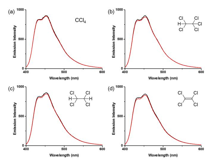
**Figure S8.** Fluorescence spectra of DPI-BP ( $5 \times 10^{-6}$  mol/L CHCl<sub>3</sub> solution) before (black) and after (red) upon addition of  $5 \times 10^{-4}$  mol/L (a) tetrachloromethane, (b) pentachloroethane, (c) 1,1,2,2-tetrachloroethane, and (d) tetrachloroethene.
