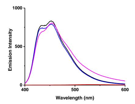
**Figure S9.** Fluorescence spectra of DPI-BP ( $5 \times 10^{-6}$  mol/L CHCl<sub>3</sub> solution) before (black) and after (red, baseline) 5.0 Gy gamma radiation. The fluorescence was recovered by addition of  $5 \times 10^{-5}$  mol/L triethylamine (blue), or 30 µL  $5 \times 10^{-3}$  mol/L NaOH EtOH:H<sub>2</sub>O = 10:1 solution, corresponding to  $5 \times 10^{-5}$  mol/L NaOH (purple).
