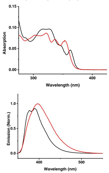
**Figure S6.** Absorption and fluorescence spectra of a CHCl<sub>3</sub> solution of PI-Ph ( $5 \times 10^{-6} \text{ mol/L}$ ) recorded before (black) and after (red) exposure to 5.0 Gy of gamma radiation.
