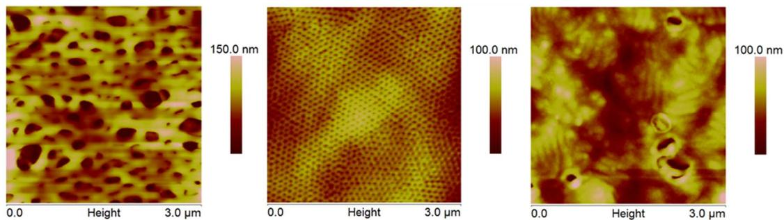
**Figure S6.** AFM height images of polymer membranes cast from a solution of 15 wt% S2VP-1 in DMF/THF: 30/70. The evaporation times are 0 sec, 15 sec, 30 sec, respectively.
