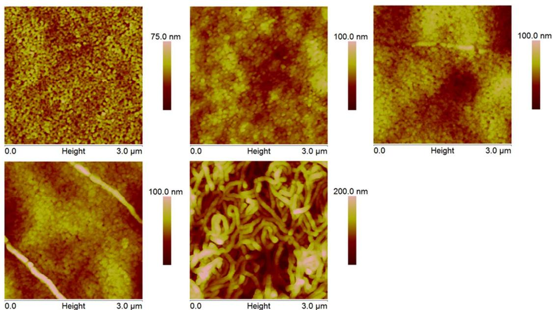
**Figure S4.** AFM height image of a polymer membranes cast from a solution of 15 wt% S2VP-1 in DMF/THF: 70/30. The evaporation times are 0 sec, 15 sec, 30 sec, 40 sec and 60 sec respectively.
