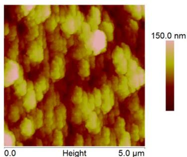
**Figure S3.** AFM height image of a polymer membrane cast from a solution of 15 wt% S2VP-1 in pure DMF after an evaporation time of 40 seconds.
