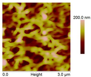
**Figure S8.** AFM height image of a polymer membrane cast from a solution of 10 wt% S2VP-1 in pure THF.
