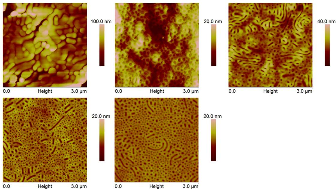
**Figure S7.** AFM height images of polymer membranes cast from a solution of 15 wt% S2VP-1 in pure THF. The evaporation times are 0 sec, 15 sec, 30 sec and 60 sec. The last image was taken from a completely dried membrane.
