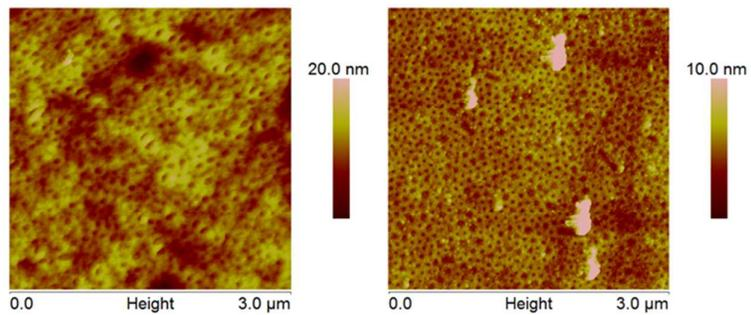
**Figure S9.** AFM height images of polymer membranes cast from a solution of 20 wt% S2VP-1 in pure THF.
