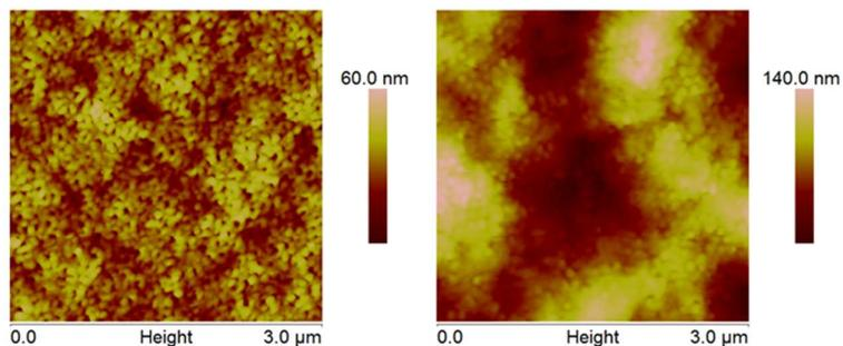
**Figure S5.** AFM height image of a polymer membranes cast from a solution of 15 wt% S2VP-1 in DMF/THF: 50/50. The evaporation times are 0 sec and 15 sec respectively.
