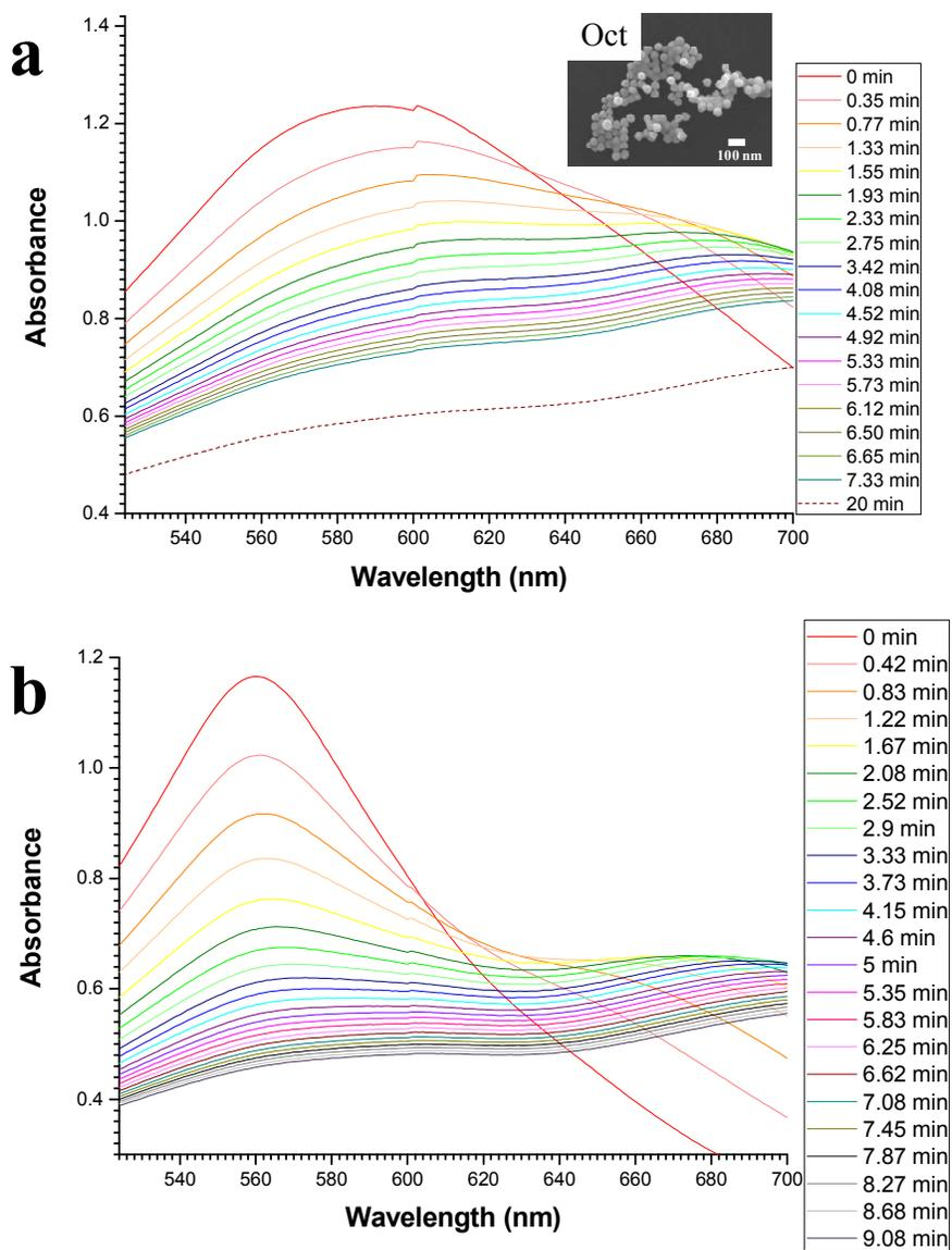
**Figure S8.** Time-dependent UV-vis absorption spectra of octahedral Au nanocrystals dispersed in (a) 0.7 and (b) 0.3 M CTAC solutions. Inset shows SEM image of the resulting aggregated octahedra.
