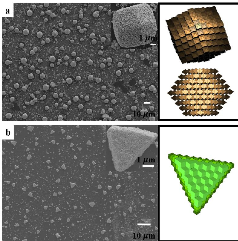
**Figure S4.** SEM images of supercrystals assembled by gold (a) octahedra and (b) rhombic dodecahedra at 90 °C by the droplet evaporation approach. Insets give the enlarged images of single supercrystals. Schematic drawings of the nanocrystal packing structures are also shown. Two viewing orientations are given for the rhombic dodecahedral supercrystals assembled from octahedral particles.
