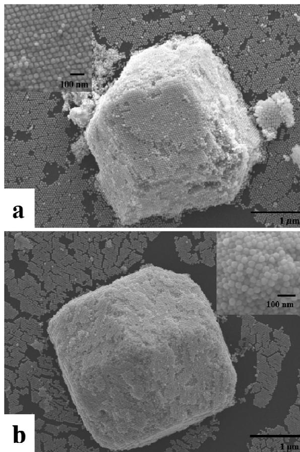
**Figure S5.** (a, b) SEM images of a single supercrystal formed through assembly of Au octahedra on an evaporating substrate at 90 °C. No interparticle fusion can be observed. Inset images show clear octahedral particles without fusion. Disk-like byproduct particles also form their own assembled structure, confirming that the particle assembly process is strongly shape-guided.
