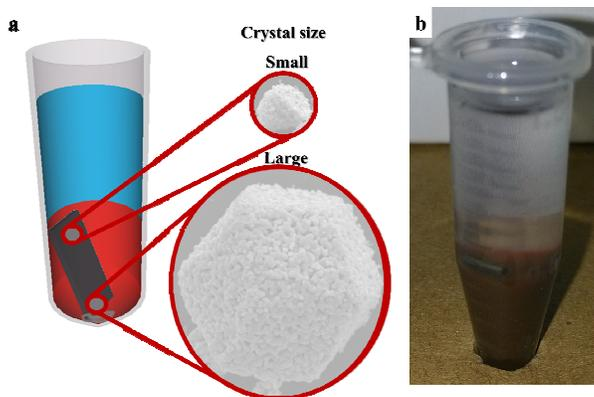
**Figure S3.** (a) Illustration of the method used to grow small and large supercrystals over a substrate. (b) Photograph showing an Eppendorf tube loaded with a slanted Si substrate. The lower layer is the gold colloidal solution, while the upper transparent layer is the CTAC solution.
