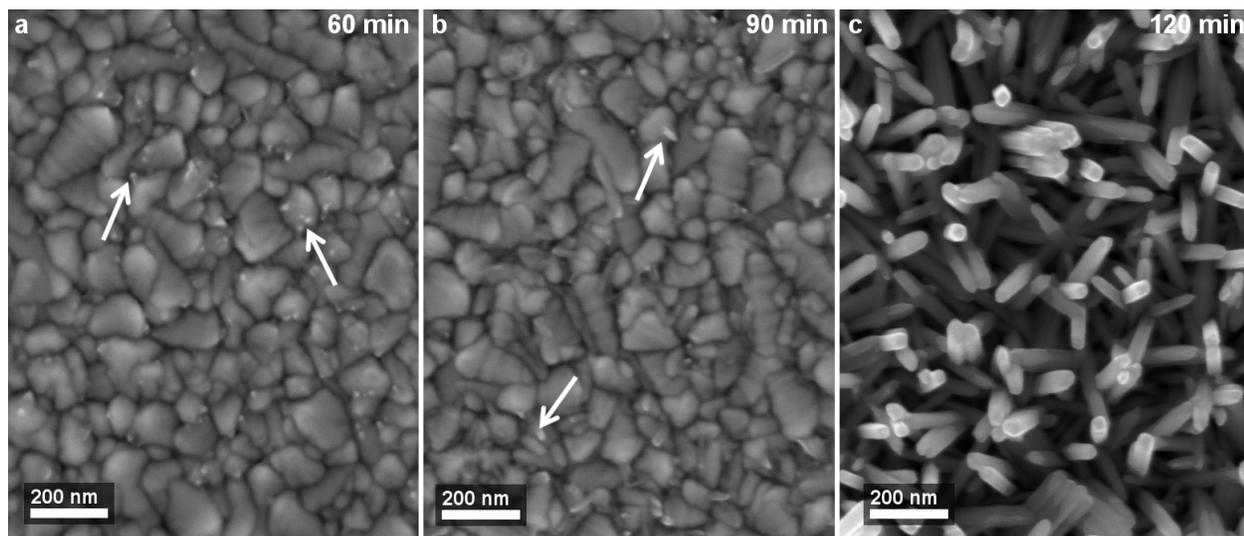
SI Figure 1: SEM images of the crystals at the start of the nanowire growth. a) After 60 minutes at 150 °C, the first crystallites can be seen on the FTO substrate. b) During the following 30 minutes, small nanowires start to develop. c) After 120 minutes, the FTO is covered by standing nanowires with an average width of 32 nm.
