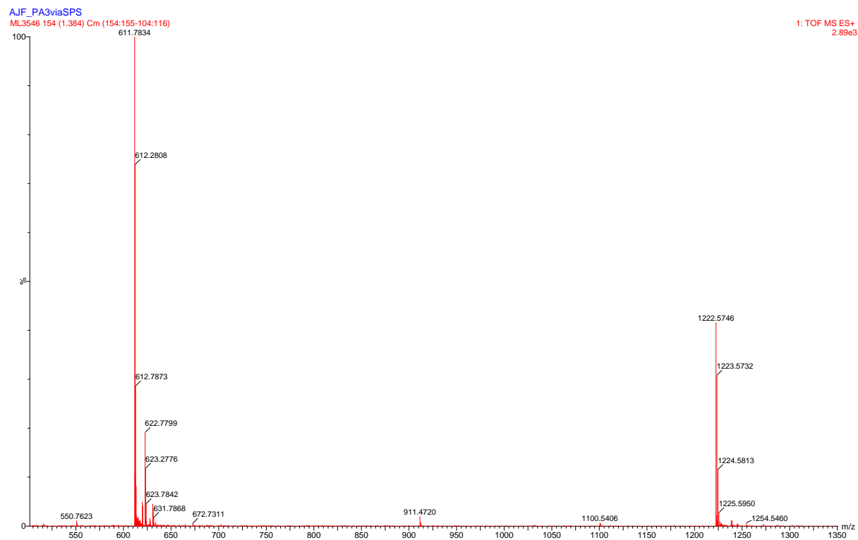
Figure S9: HRMS of polyamide ( 19a ). Key peaks shown are [M+H]^+ at 1222.5746, [M+2H]^{2+} at 611.7834, [M+H+Na]^{2+} at 622.7799.
