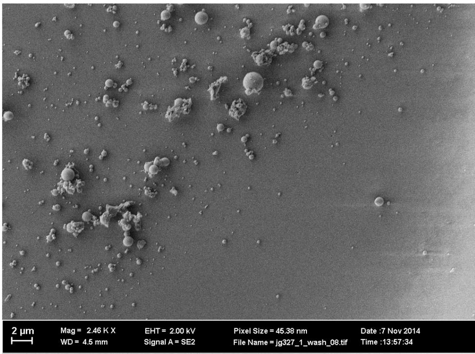
Figure S10: SEM/EDX data for immobilization of SH50 particles on stainless steel surfaces.
