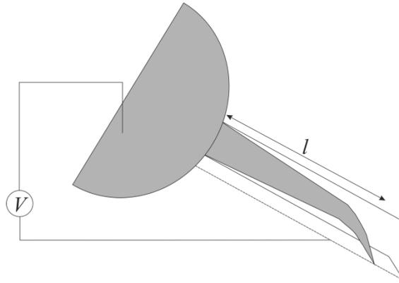
Figure S1. Schematic diagram of the experimental set-up showing a reservoir drop and a drawn liquid filament in a triangular groove. The top electrode was immersed in the reservoir drop and the bottom electrode was connected to underlying conducting silicon substrate.
