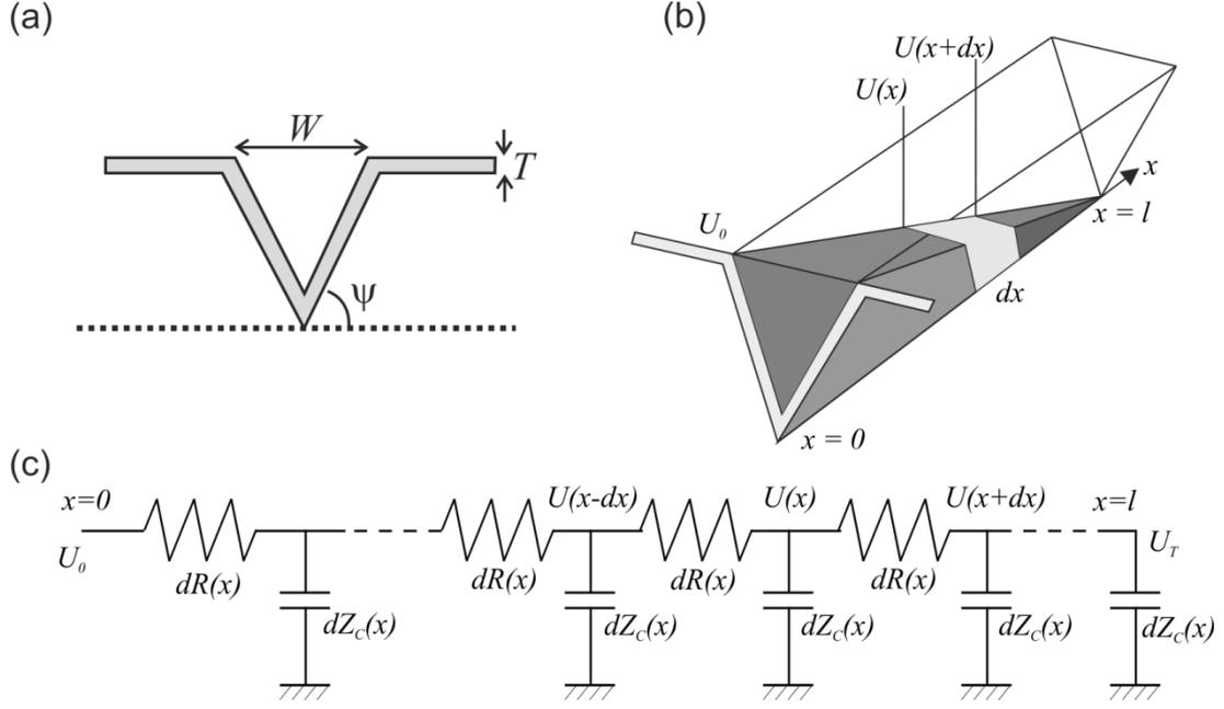
Figure S1. (a) Sketch of a triangular groove showing all parameters, (b) sketch of a liquid filament with linearly decreasing width in a triangular groove and (c) equivalent electrical circuit for a liquid filament in a triangular groove.
