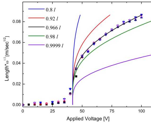
Figure S2. Plot of the scaled experimental data with the solution of linearly decreasing filament model for different values of  $x$  around  $x = l$  showing that  $x = 0.966l$  fits the best.
