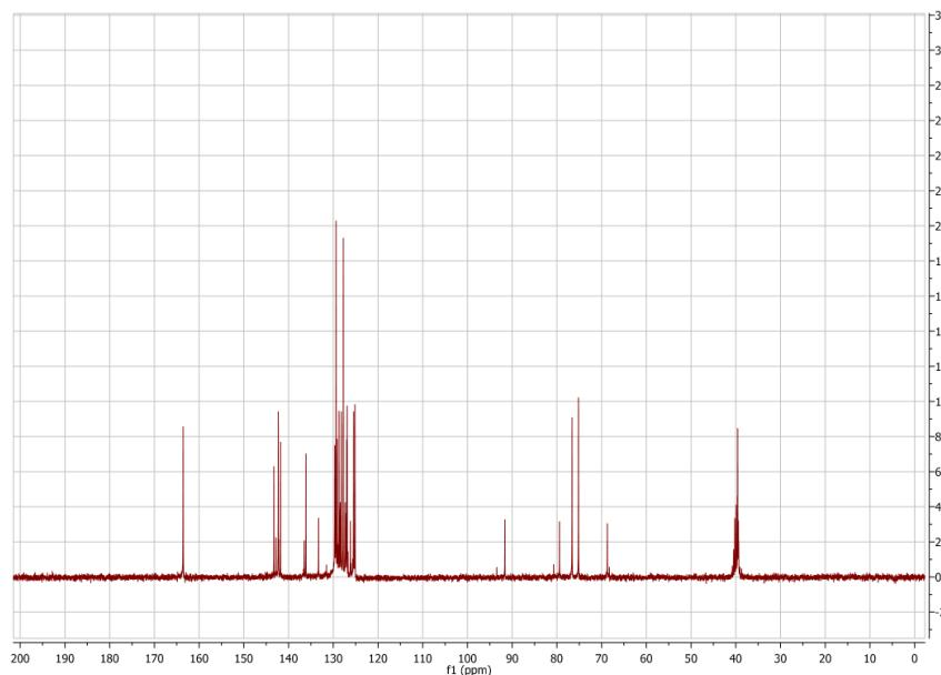
**Figure S12.** (a) ESI-MS and (b) <sup>13</sup>C NMR spectra of **P2** in DMSO- $\delta_6$ .
