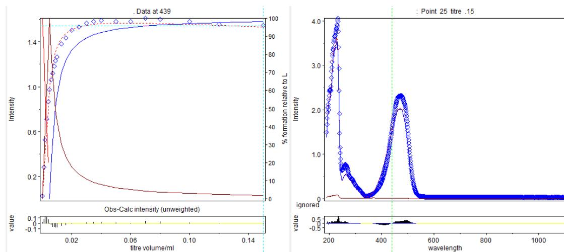
**Figure S4A.** Spectrophotometric for  $4 \times 10^{-5}$  M **P1** with (0 to  $5.6 \times 10^{-4}$  M)  $\text{SnPh}_2^{2+}$  in acetonitrile : water (4 : 96, v/v) solution. The maroon line accounts for  $[\text{P1} : \text{Sn}] = 2 : 1$  complex, observed in a); while the blue line for 1 : 1 complex observed in b).
