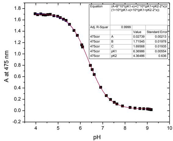
**Figure S3.** Spectrophotometric pH titration of **P1** in using hexadecyltrimethylammonium chloride (HTAB, 5 mM) and *N*-Cyclohexyl-2-aminoethanesulfonic acid (CHES) buffer at pH 9.2
