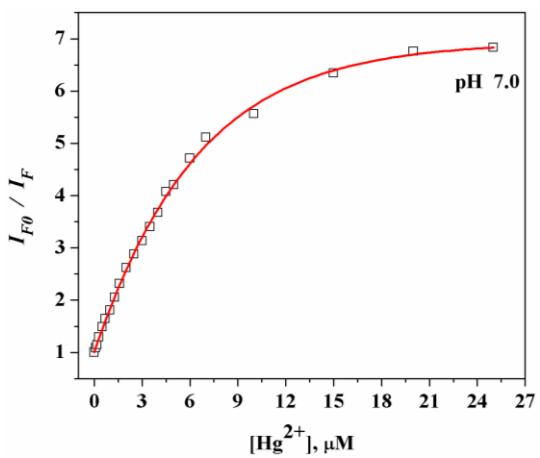
**Figure S7.** The concentration profile of the quenching effect of  $\text{Hg}^{2+}$  (Stern-Volmer plot) at pH 7.0
