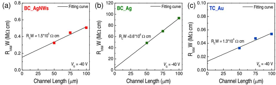
**Figure S1** Channel width-normal total resistance as a function of channel length for pentacene OFETs with (a) bottom contact AgNWs, (b) bottom contact Ag, and (c) top-contact Au as source/drain electrodes at  $V_G = -40$  V.
