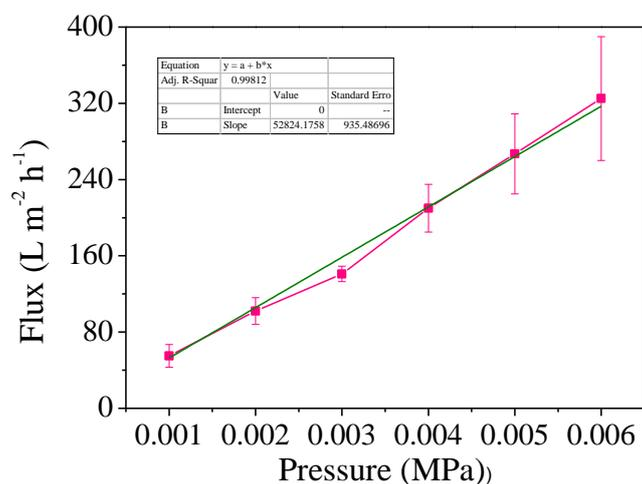
**Figure S8.** The flux of CNT hollow-fiber membranes as a function of pressure.
