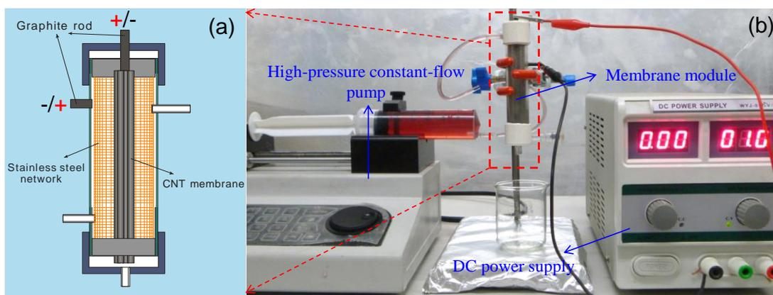
**Figure S6.** (a) Schematic illustration of the membrane module. (b) The experimental setup used in this work.
