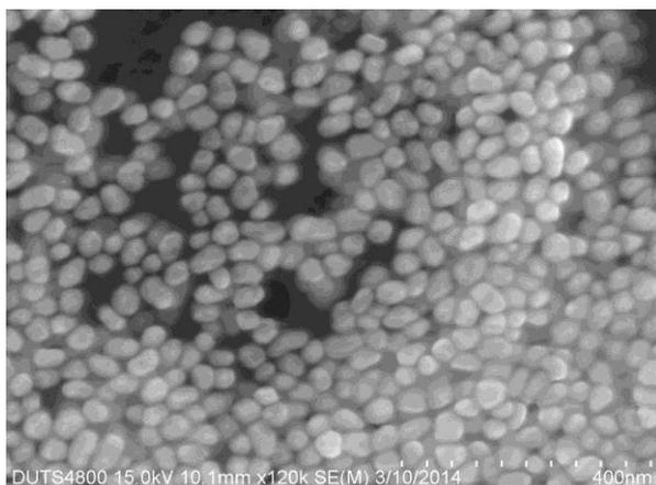
**Figure S2.** Scanning electron microscope image of 40 nm GNPs.
