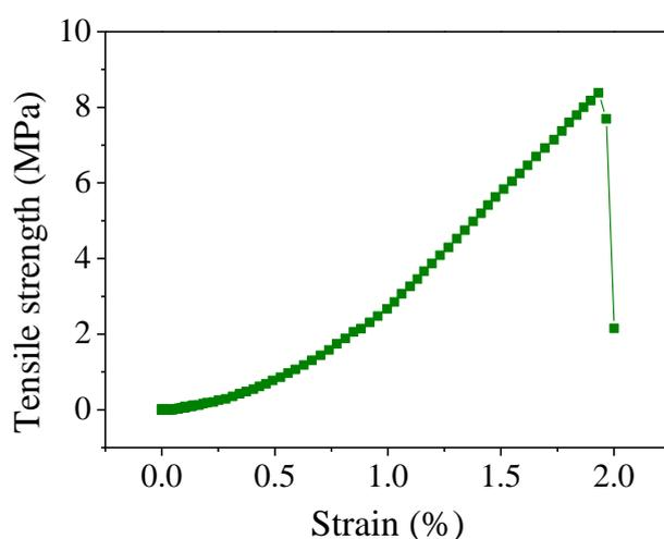
**Figure S3.** Typical stress-strain curve of prepared CNT hollow-fiber membrane.
