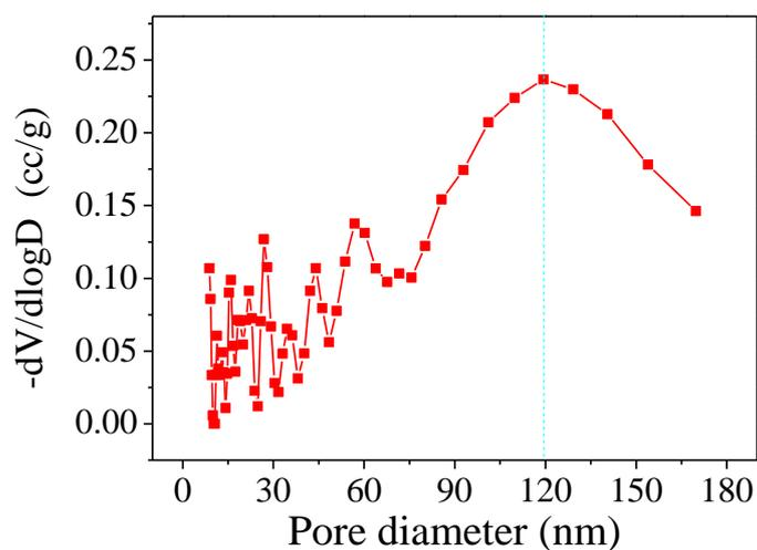
**Figure S7.** The pore size distribution of CNT hollow-fiber membranes. This characterization is performed using a mercury porosimeter (Quantachrome PoreMaster-60GT).
