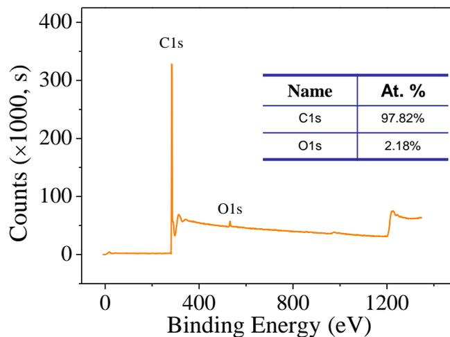
**Figure S5.** The X-ray photoelectron spectroscopy analysis of CNT hollow-fiber membranes after calcination in a mixture flow of Ar (40 sccm) and H<sub>2</sub> (10 sccm) at 1000 °C for 2 h.
