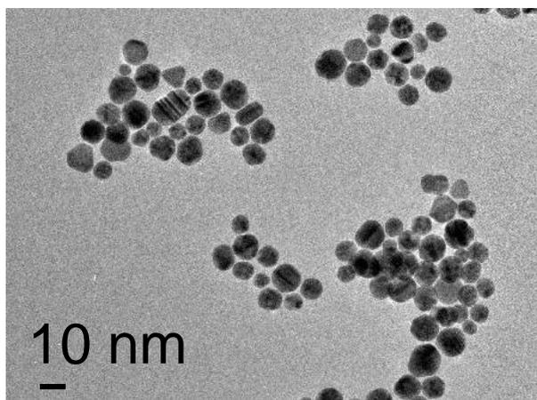
**Figure S1.** Transmission electron microscope image of 10 nm GNPs.
