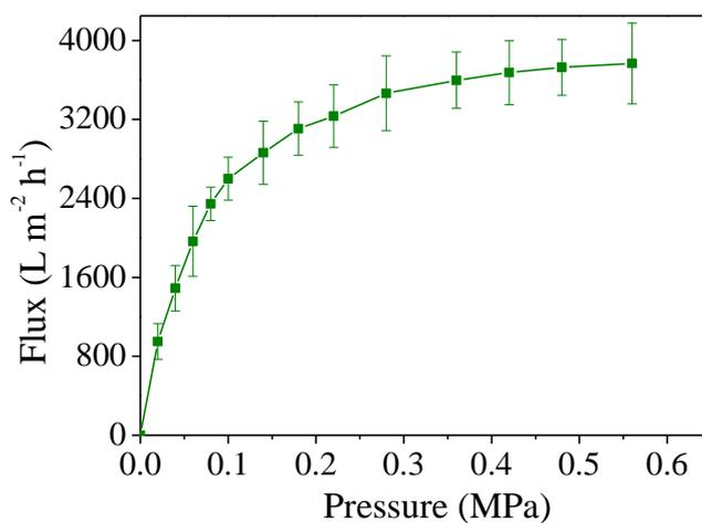
**Figure S4.** The transmembrane flux as a function of pressure.
