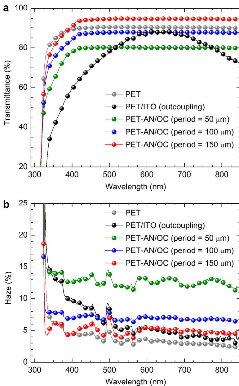
**Figure S2.** Comparison of optical properties of various PET-AN/OCs with the bare PET and ITO-coated PET (ITO/PET) with a moth-eye antireflection coupling layer. (a) Transmission spectra and (b) haze values of PET-AN/OCs with various hexagonal periods as a function of wavelength. The haze values were obtained by collecting the total transmittance and the specular transmittance with in integrating sphere [haze = (total transmittance - specular transmittance)/total transmittance].
