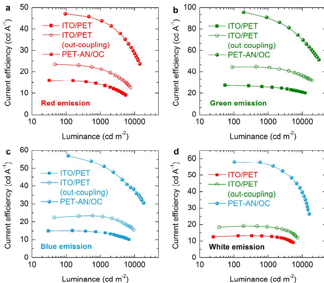
**Figure S4.** Current efficiencies as a function of luminance for FOLEDs using various plastic substrates with (a) red, (b) green, (c) blue, and (d) white emissions.
