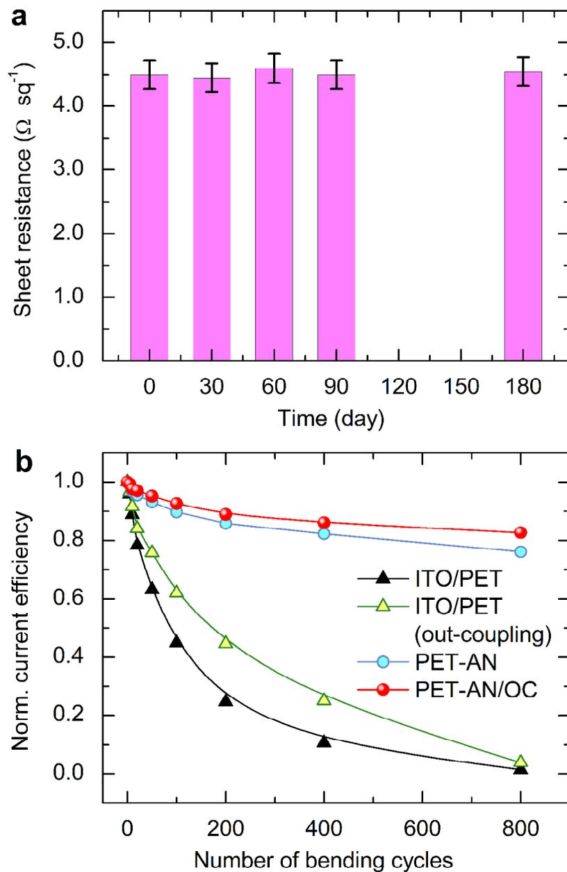
**Figure S3.** Comparison of the storage and mechanical stabilities of PET-AN/OCs. (a) The storage stability of PET-AN/OCs exposed to the air without any protection. (b) Normalized current efficiencies of green FOLEDs using various substrates are compared during the repeated bending, where the tests were conducted by repeatedly bending the substrates to a radius of curvature of about 6 mm at a constant current density of  $15 \text{ mA cm}^{-2}$ .
