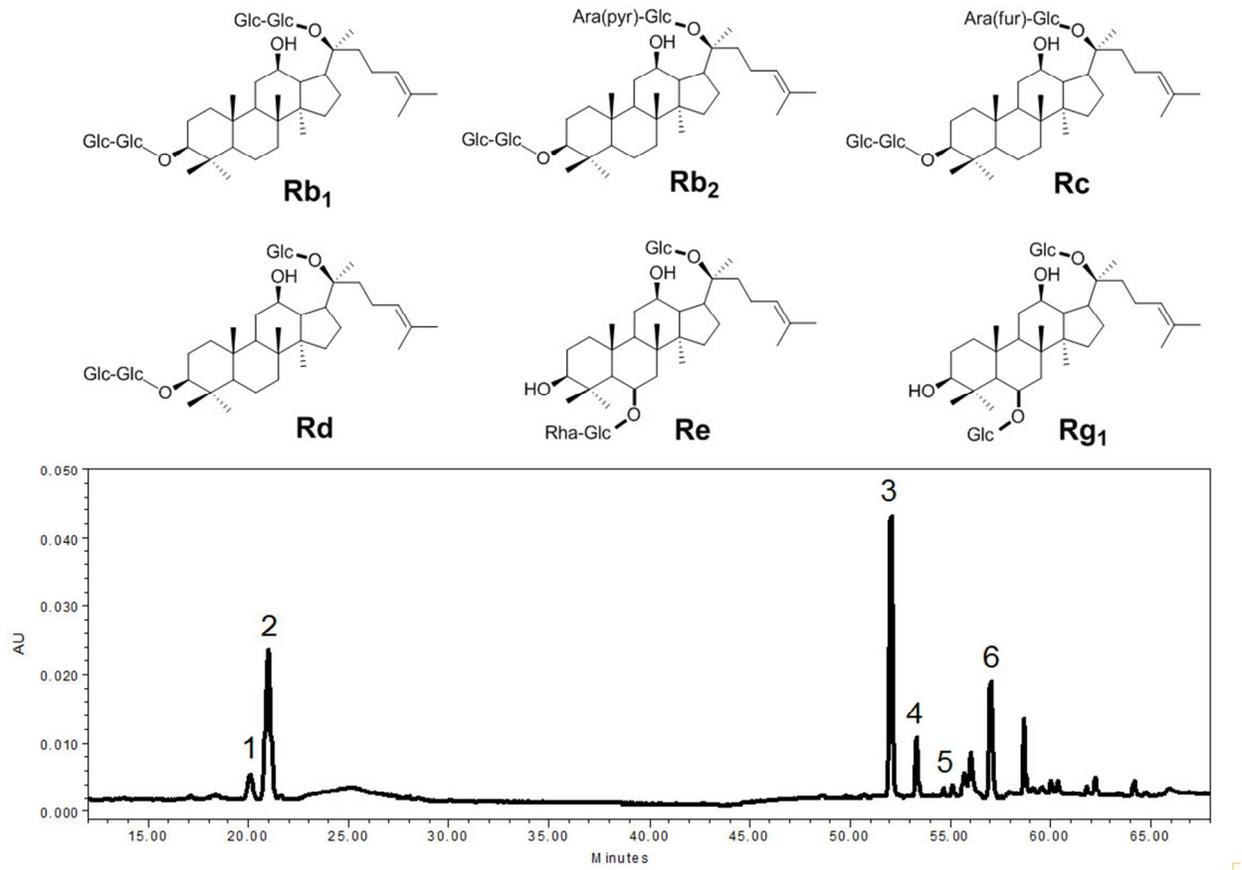
**Supplementary Figure 1.** HPLC analysis of American ginseng extract. **(A)**, Chemical structures of measured ginsenosides; **(B)**, HPLC chromatogram of American ginseng recorded at 202 nm. Ginsenoside peaks: 1, Rg<sub>1</sub>; 2, Re; 3, Rb<sub>1</sub>; 4, Rc; 5, Rb<sub>2</sub>; 6, Rd.
