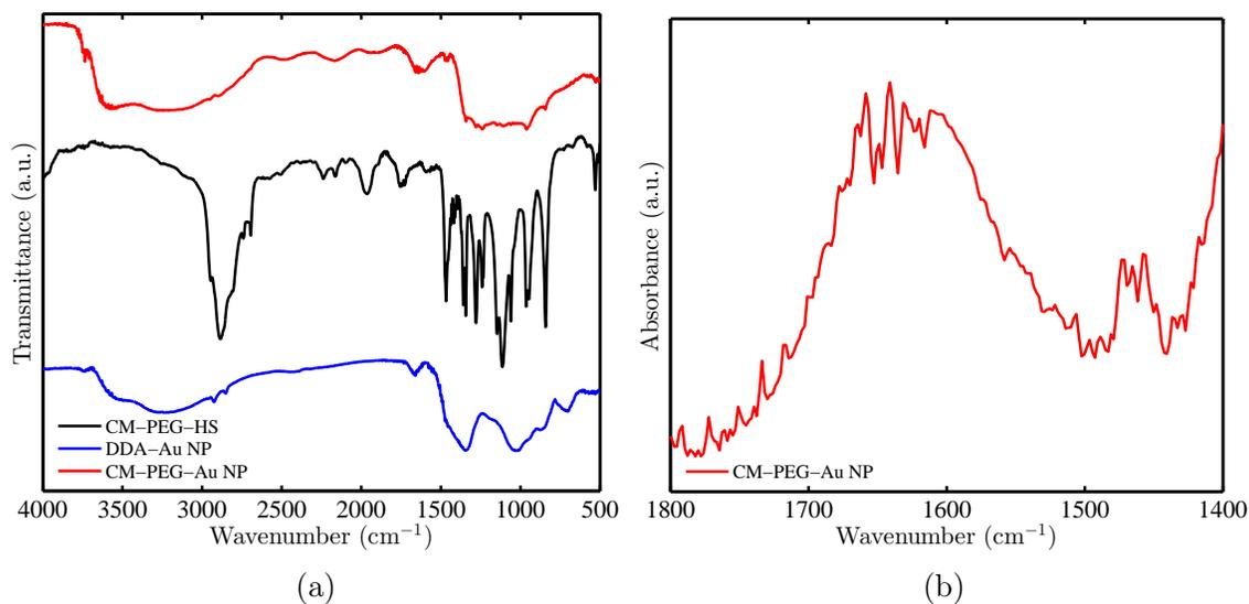
Figure 2: (a) DRIFT-FTIR transmittance of CM-PEG-HS (black), DDA-Au NPs (blue), and CM-PEG-Au NPs (red); (b) DRIFT-FTIR absorbance of CM-PEG-Au NPs.
