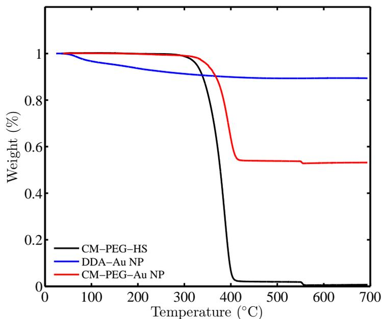
Figure 5: TGA of CM-PEG-HS (black), DDA-Au NPs (blue) and CM-PEG-Au NPs (red).
