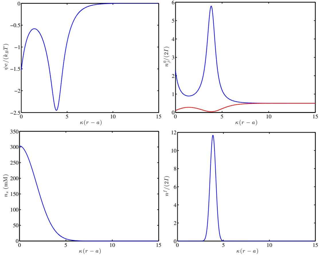
Figure 10: Radial profiles of electrostatic potential  $\psi$  (top left), equilibrium mobile ion densities  $n_j^0$  (top right), segment (5kPEG-chain) density  $n_s$  (bottom left), and fixed charge density  $n_j^f$  (bottom right) for SH-PEG-COOH functionalized NPs ( $a = 10$  nm,  $\chi = 1$ ) at  $I = 20$  mM.
