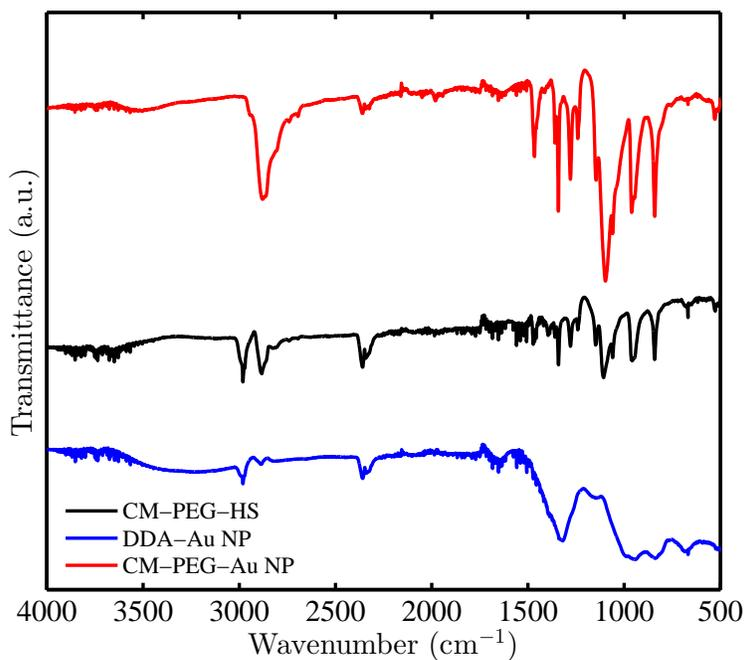
Figure 1: Diamond ATR-FTIR transmittance of CM-PEG-HS (black), DDA-Au NPs (blue), and CM-PEG-Au NPs (red).
