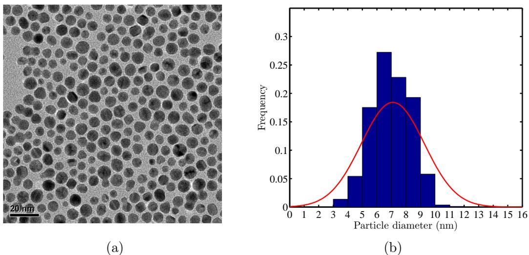
Figure 3: TEM micrograph (a) and size histogram (b) of DDA-Au NPs.
