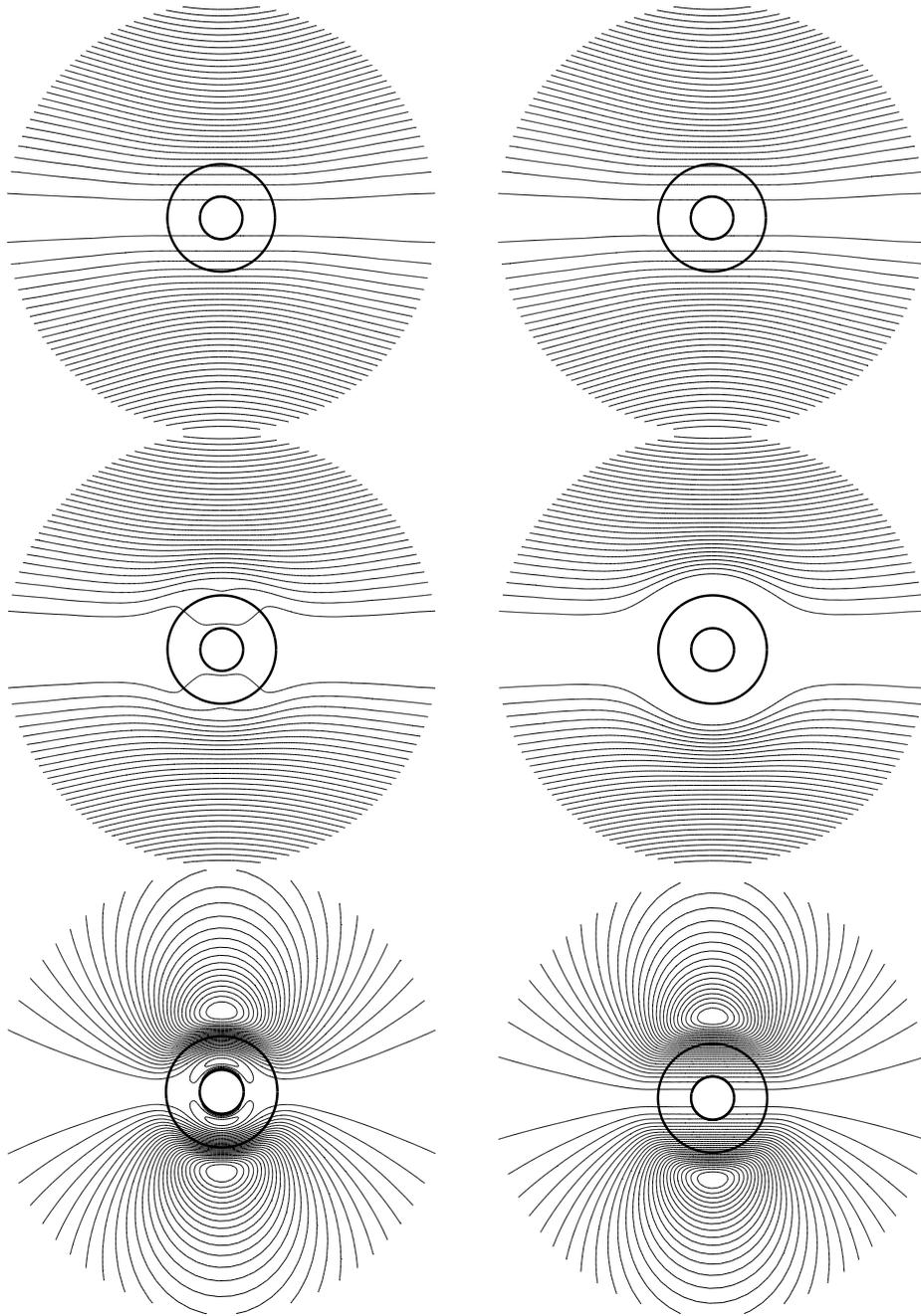
Figure 9: Streamlines for CM-5kPEG-Au NPs with  $I = 100$  mM ( $L \approx 5$  nm) for uncharged (left) and charged (right) coronas: translation in the absence of an electric field (diffusion, top); stationary particle in an electric field (electroosmosis, middle); translation under an electric field (force-free electrophoresis, bottom). Inner and outer circles identify the Au core and nominal coating periphery.
