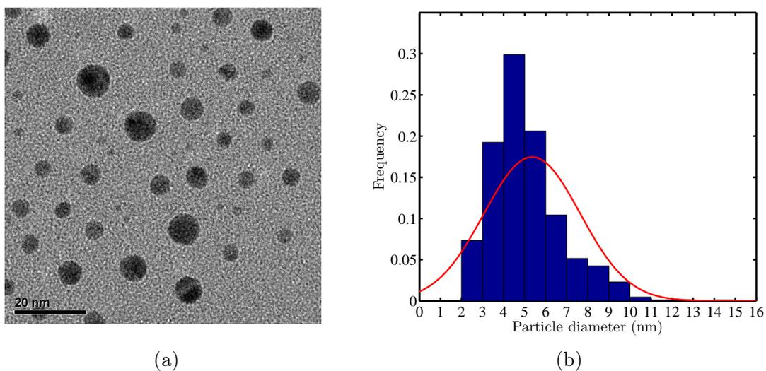
Figure 4: TEM micrograph (a) and size histogram (b) of CM-PEG-Au NPs.
