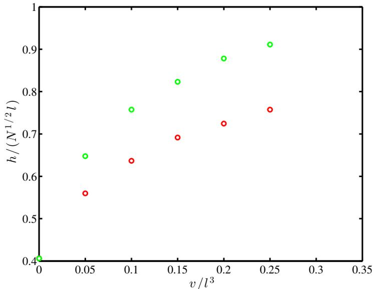
Figure 8: Self-consistent-field computation of the layer thickness  $h/(N^{1/2}l)$  versus the dimensionless excluded volume parameter  $v/l^3$  for uncharged excluded-volume chains end-grafted to a nanoparticle (core radius  $a = 2.7$  nm)  $l = 0.6$  nm) (red) and a flat plate (green). Computations with dimensionless grafting density  $\gamma l^2 = 0.57$  and chain length  $N = 83$  ( $N^{1/2}l \approx 5.5$  nm).
