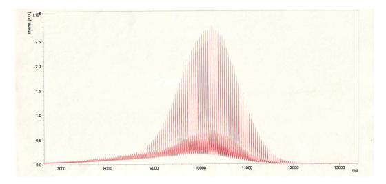
Figure S1: A MALDI-TOF spectrum of the tetra-amine-terminated PEG (Mw: 10 kg/mol, Mw/Mn = 1.05).
