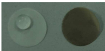
Figure S8. Contact angle compared between PE bare separator and PD modified separator by adding 0.04ml electrolyte.
