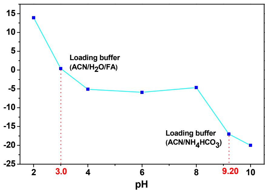
**Figure S2** Dependence of zeta spectra of Fe<sub>3</sub>O<sub>4</sub>-DA-Maltose NPs on the change of pH.
