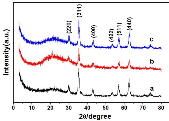
**Figure S1** XRD patterns of  $\text{Fe}_3\text{O}_4$  (a),  $\text{Fe}_3\text{O}_4$ -DA-N<sub>3</sub> (b) and  $\text{Fe}_3\text{O}_4$ -DA-Maltose (c) NPs.
