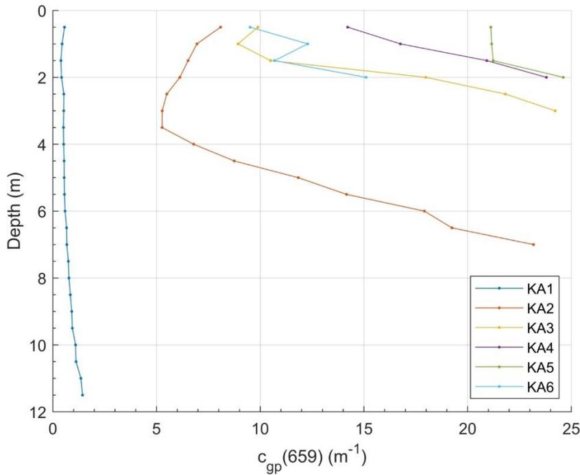
**Figure 4.** Attenuation profiles at 659 nm measured by a Wetlabs ac-s meter. These 6 stations were measured on the North Slope near Kaktovik Ak during the Jago River transect (KA2018).
