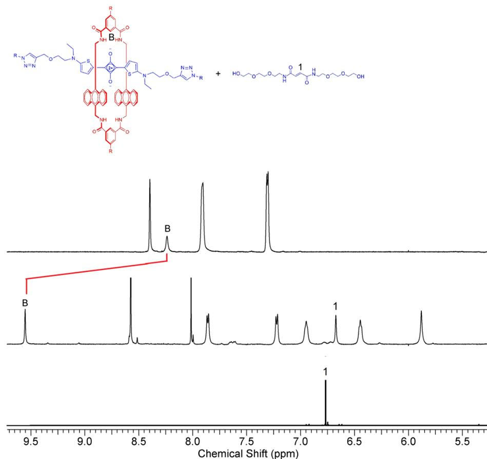
Figure S21: Partial  $^1\text{H}$  NMR (600 MHz,  $D_2O$ ,  $25\text{ }^\circ\text{C}$ ) of (top) **M2**:**F1** (2.0 mM); (middle) **M2**:**F1** (2.0 mM) treated with **S3** (2.0 mM) which displaced **F1**; (bottom) fumaride **F1** (2.0 mM). Red line indicates change in chemical shift for **M2** peak B upon displacement of **F1** by **S3**.
