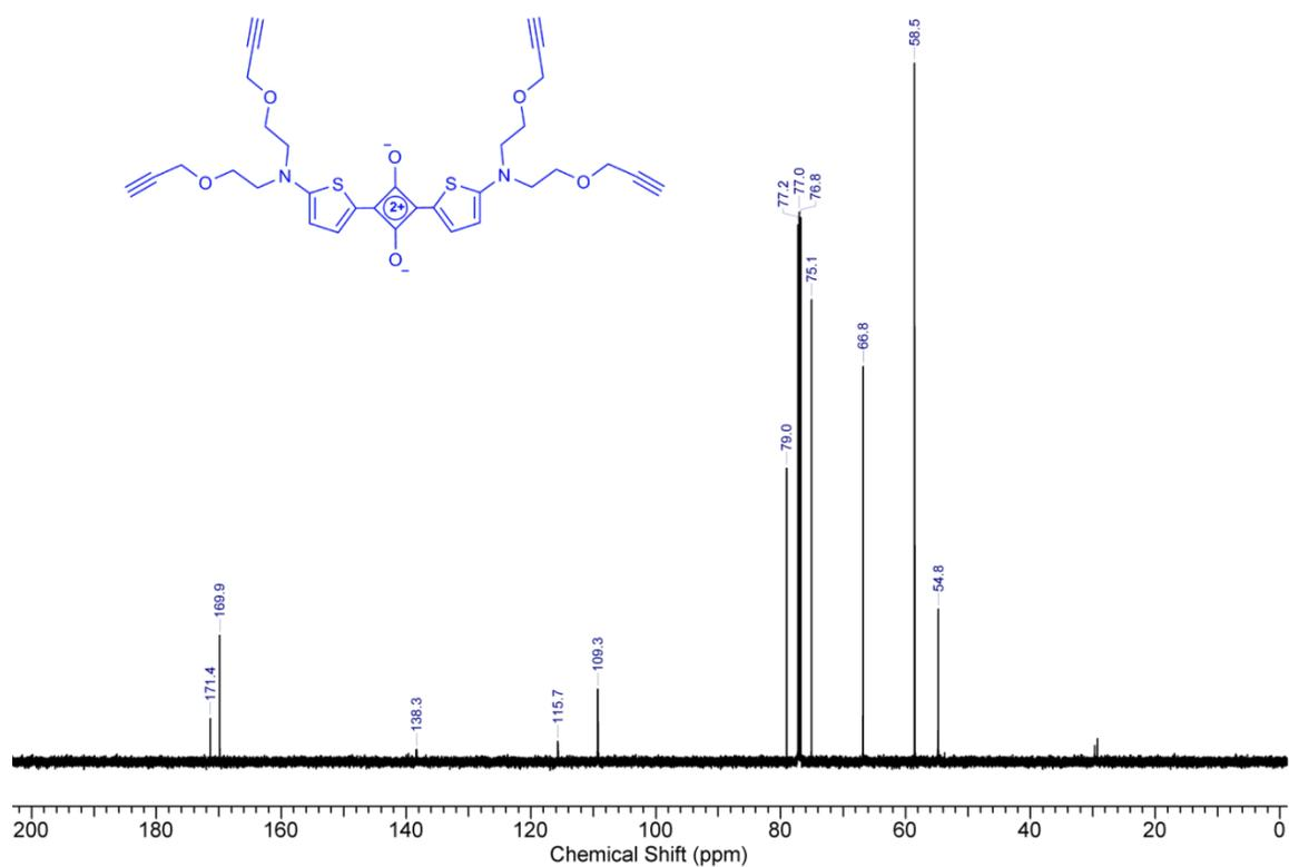
Figure S43:  $^{13}\text{C}$  NMR (150 MHz,  $\text{CDCl}_3$ , 25  $^\circ\text{C}$ ) spectrum of squaraine dye **3**.
