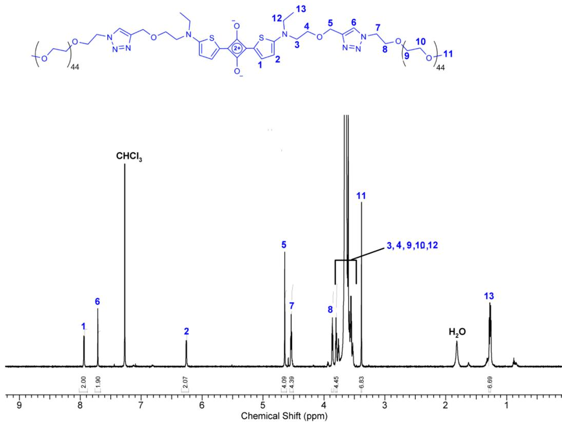
Figure S41:  $^1\text{H}$  NMR (600 MHz,  $\text{CDCl}_3$ , 25  $^\circ\text{C}$ ) spectrum of squaraine dye **S3**.
