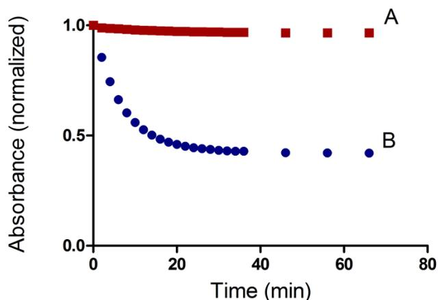
Figure S11: Change in absorbance of maxima band for solutions of A) complex **M2**⊃**S3** (5.0 μM **S3**, 7.5 μM **M2**) or B) squaraine dye **S3**, in the presence of external nucleophile Na<sub>2</sub>S (10 mM) in water at 25°C.
