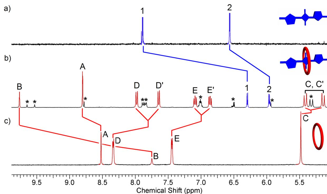
Figure S6: Partial  $^1\text{H-NMR}$  (600 MHz,  $\text{CD}_3\text{OD}$ , 25  $^\circ\text{C}$ ) of a) **S1** (2.0 mM); b) **M2** (2.0 mM); and c) **M2:S1** (2.0 mM). Red and blue lines indicate major changes in chemical shift upon complexation. \*indicates signals corresponding to the minor **M2:S1** complex with **S1** encapsulated as *cis* conformer (*trans:cis* ratio for encapsulated **S1** ~3:1).
