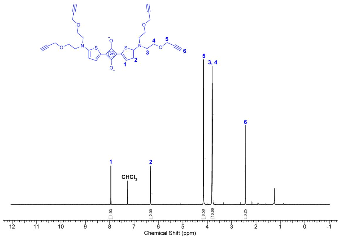
Figure S42:  $^1\text{H}$  NMR (500 MHz, CDCl<sub>3</sub>, 25 °C) spectrum of squaraine dye **3**.
