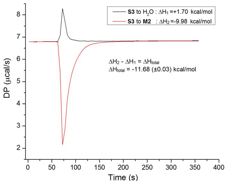
Figure S25: ITC single injection of **S3** into H<sub>2</sub>O or an aqueous solution containing **M2** (50 μM, 27 °C) enabled determination of the enthalpy of complexation.
