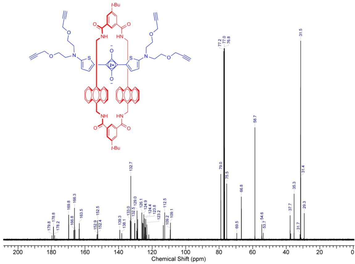
Figure S45:  $^{13}\text{C}$  NMR (150 MHz,  $\text{CDCl}_3$ , 25 °C) spectrum of squaraine dye **SR1**.
