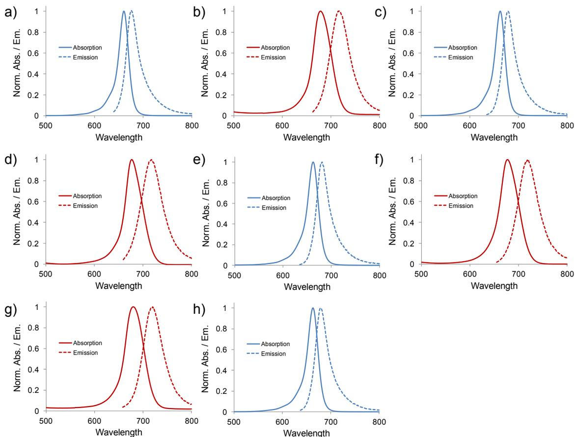
**Figure S1:** Absorption and emission maxima of a) squaraine dye **S1**; b) complex **M1>S1**; c) squaraine dye **S2**; d) complex **M1>S2**; e) squaraine dye **S3**; f) complex **M1>S3**; g) squaraine rotaxane **SR1**; and h) squaraine dye **S4** in  $\text{CHCl}_3$  (3.0  $\mu\text{M}$ ).
