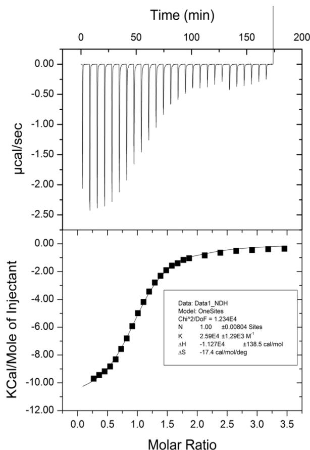
Figure S24: ITC titration of **F1** into an aqueous solution containing **M2** at 27  $^{\circ}\text{C}$ .
