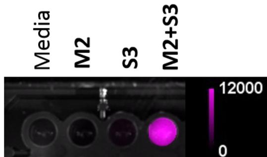
Figure S37. Image of a microwell plate using a CCD camera and an illumination filter set that allowed blue excitation (410/10 nm) and captured red emission (700/17.5 nm). Each microwell (4 mm diameter) contained a solution of additive (10  $\mu\text{M}$ ) in culture media (200  $\mu\text{L}$ ), and the image is an overlay of a photograph and a fluorescence intensity pixel map. The fluorescence intensity bar is in arbitrary units.
