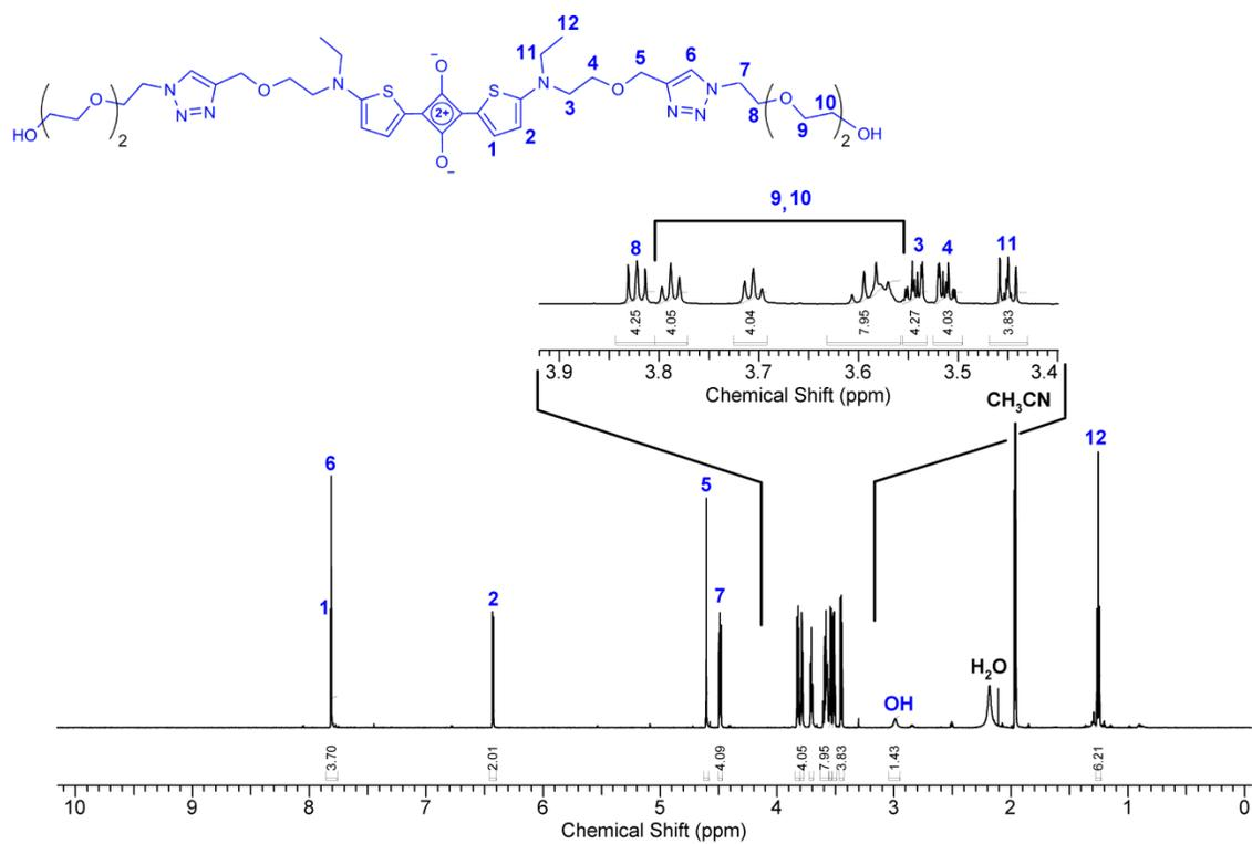
Figure S40:  $^1\text{H NMR}$  (500 MHz,  $\text{CD}_3\text{CN}$ , 25 °C) spectrum of squaraine dye **S2**.
