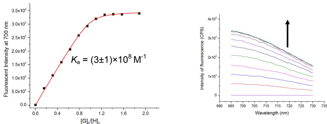
Figure S22: Determination of  $K_a$  by the competitive displacement of **F1** from **M2:F1** by addition of squaraine **S2** to a mixture of **M2+ F1** (**F1:M2** molar ratio was 100:1) in  $\text{H}_2\text{O}$  at  $20^\circ\text{C}$ .
