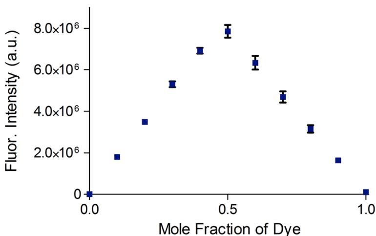
Figure S10: Job Plot indicating 1:1 binding between **S3** and **M2** ([**S3**+**M2**] = 2.0  $\mu\text{M}$ ,  $\text{H}_2\text{O}$ , 25  $^{\circ}\text{C}$ , Excitation = 710 nm, Emission = 725 nm).
