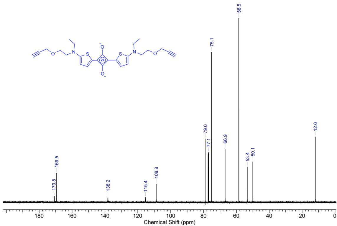
Figure S39:  $^{13}\text{C}$  NMR (150 MHz,  $\text{CDCl}_3$ , 25 °C) spectrum of squaraine dye **S1**.
