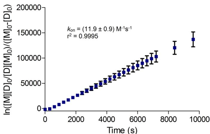
Figure S29: Second-order kinetic plot for the rate of association between **S3** and **M1** in  $\text{CHCl}_3$  at  $20^\circ\text{C}$ .  $N = 3$ .
