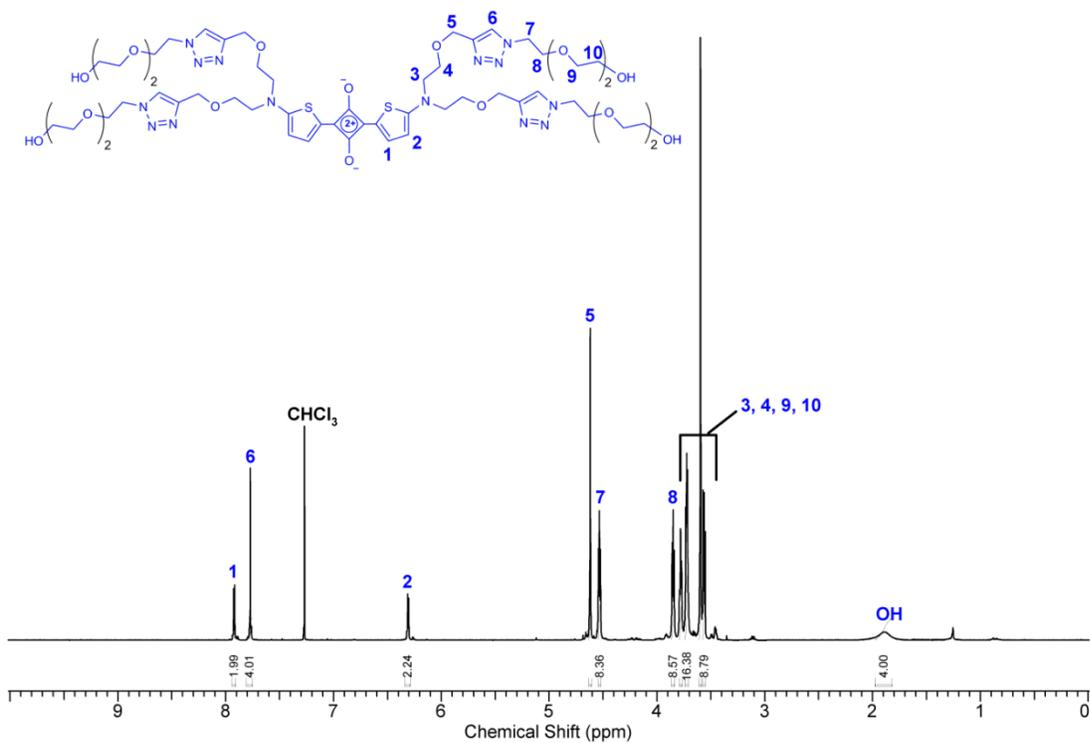
Figure S46: <sup>1</sup>H NMR (500 MHz, CDCl<sub>3</sub>, 25 °C) spectrum of squaraine dye **S4**.
