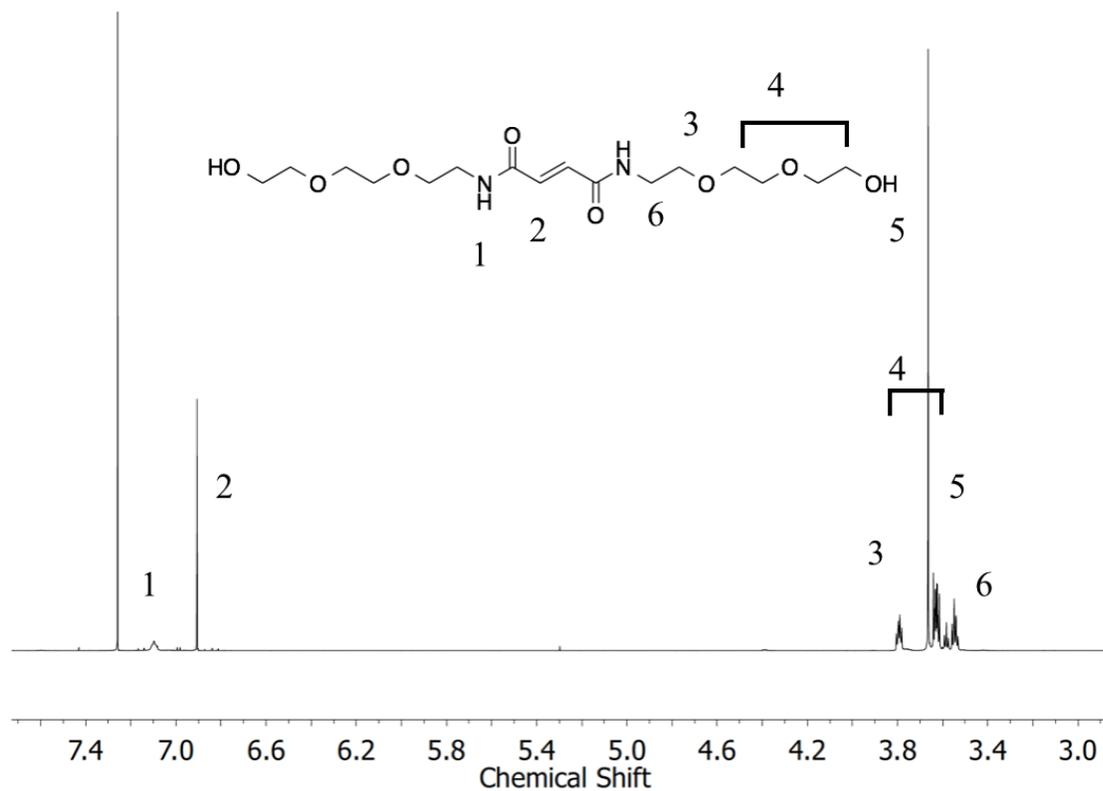
Figure S47: <sup>1</sup>H NMR (500 MHz, CDCl<sub>3</sub>, 25 °C) spectrum of fumaride **F1**.
