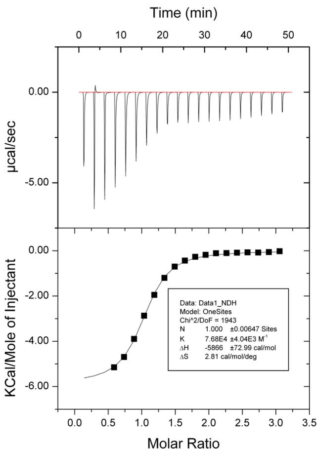
Figure S27: ITC titration of **N1** into an aqueous solution containing **M2** in  $\text{H}_2\text{O}$  at 27  $^{\circ}\text{C}$ .
