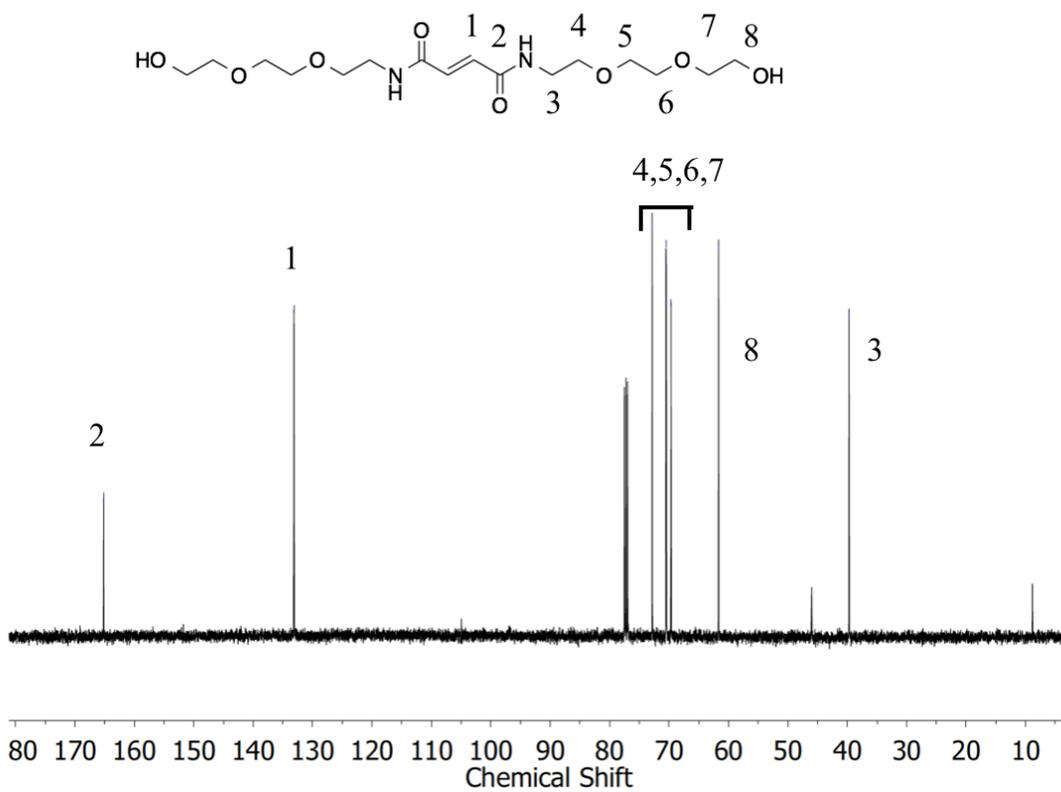
Figure S48:  $^{13}\text{C}$  NMR (150 MHz,  $\text{CDCl}_3$ , 25 °C) spectrum of fumaride **F1**.
