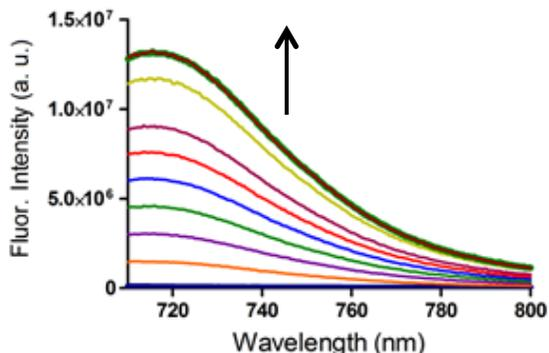
Figure S9: Fluorescence emission of **S3** (3.0  $\mu\text{M}$ ) upon addition of **M2** (up to 2 mol. equiv.) showing dramatic turn-on effect (25  $^{\circ}\text{C}$ ,  $\text{H}_2\text{O}$ , Excitation = 690 nm).
