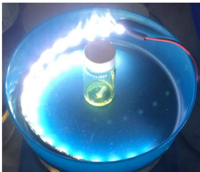
**Figure SI 2.** Photograph of experimental setup for polymerizations conducted using LED irradiation.
