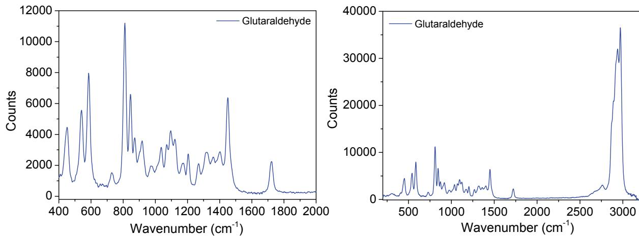
**Figure S2.** Raman spectra of glutaraldehyde. Spectra was collected using a 532 nm CW laser (250 mW) in a 90° scattering configuration. The analyzer was set with the polarization plane parallel to that of the incoming laser.
