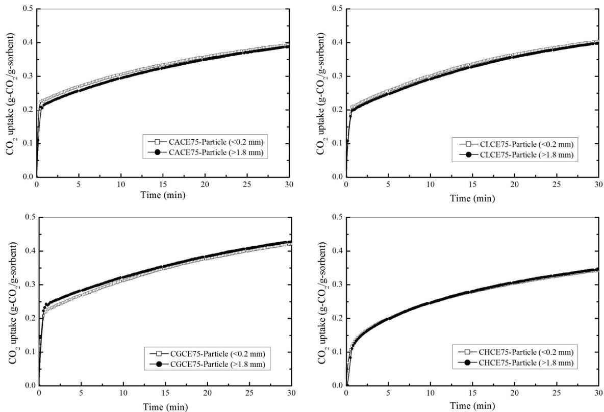
Figure S1. CO<sub>2</sub> uptake profile of different sized sorbent pellets as a function of time in the first cycle. Calcination was performed at 900 °C, with 100% N<sub>2</sub> for 10 min; carbonation was performed at 650 °C with 15% CO<sub>2</sub> for 30 min.
