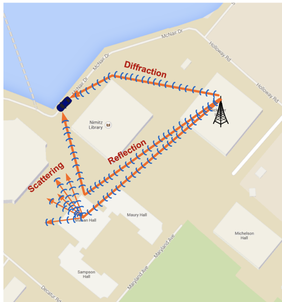
Figure 4.3 Propagation modes of Reflection, Diffraction and Scattering (USNA, 2016)
