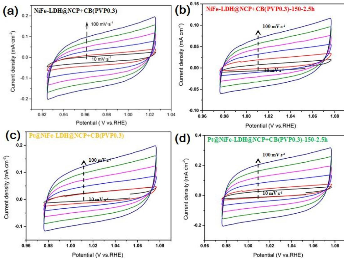
**Figure S4.** (a) CVs of the NiFe-LDH@NCP+CB (PVP 0.3), (b) NiFe-LDH@NCP+CB(PVP 0.3)-150-2.5h, (c) Pt@NiFe-LDH@NCP+CB(PVP 0.3), and (d) Pt@NiFe-LDH@NCP+CB(PVP 0.3)-150-2.5h at different scan rates of 10, 20, 40, 60, 80 and 100  $\text{mV s}^{-1}$ .
