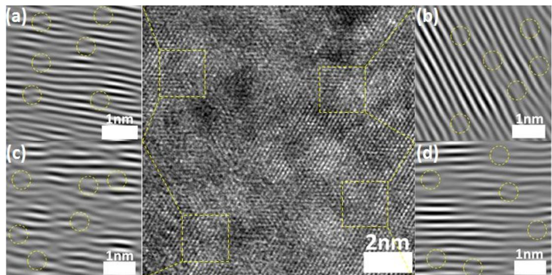
**Figure S2.** TEM images of defects and dislocations of Pt@NiFe-LDH@NCP+CB(PVP 0.3)-150-2.5h, and after Fourier transform.
