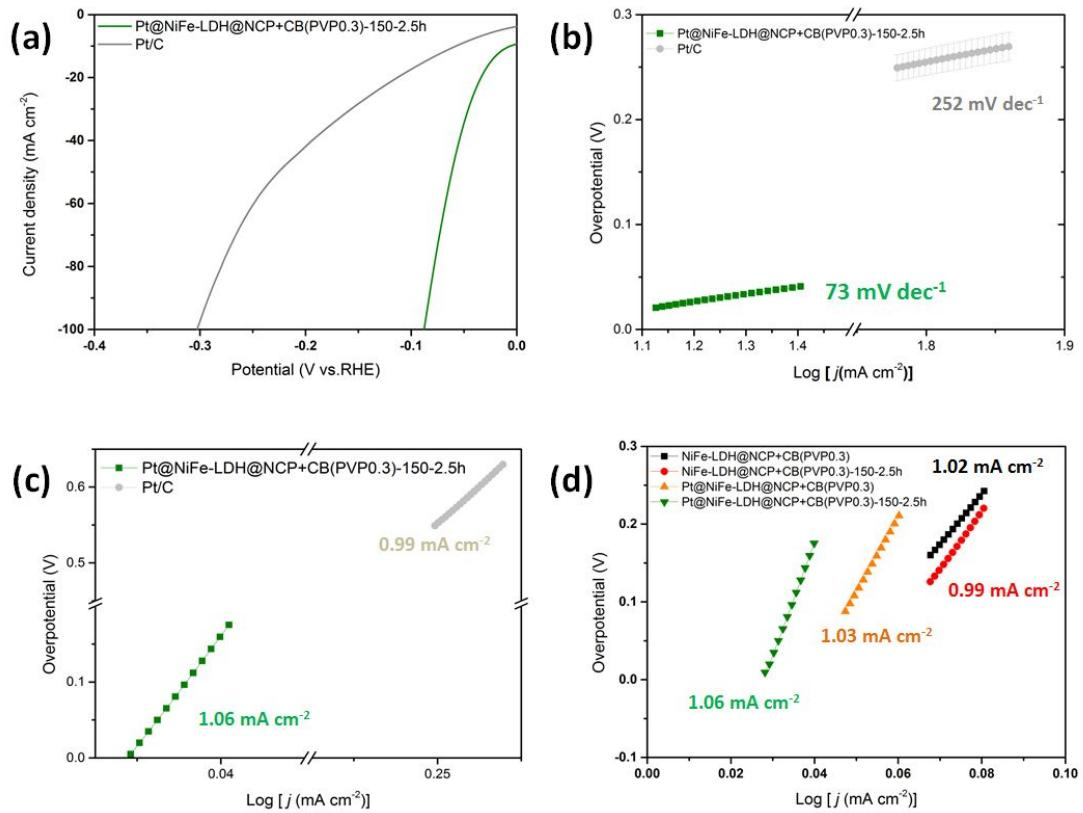
**Figure S5.** (a) HER LSV curve of the Pt@NiFe-LDH@NCP+CB(PVP 0.3)-150-2.5h and Pt/C, (b) Tafel plots , and (c,d) Exchange current density.
