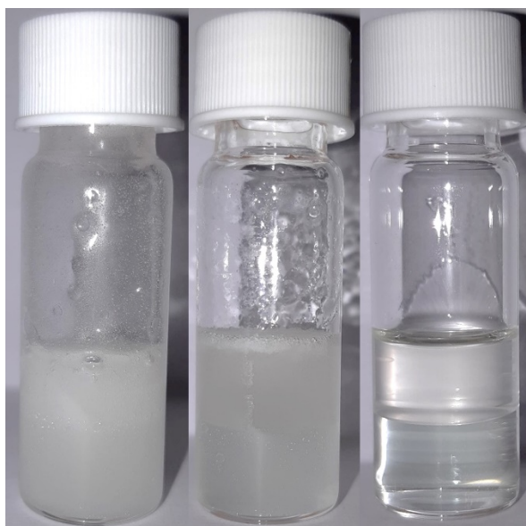
Figure S2: Pictures of the phase disengagement process of undiluted [A336][HSO_4] and the synthetic germanium containing leachate after equilibration. Left: directly after shaking.
