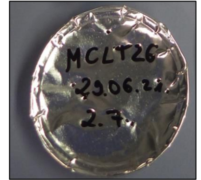
Sealed AOM filter (drying: 50 °C, 48 h)
