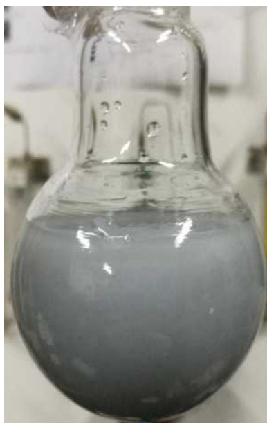
Figure S1. The picture of Sb powders dispersed in \text{H}_2\text{SO}_4 solvent ( 8.0 \text{ mg mL}^{-1} ) with continuous stirring (400 r/min) at 298 K after 12.0 h.
