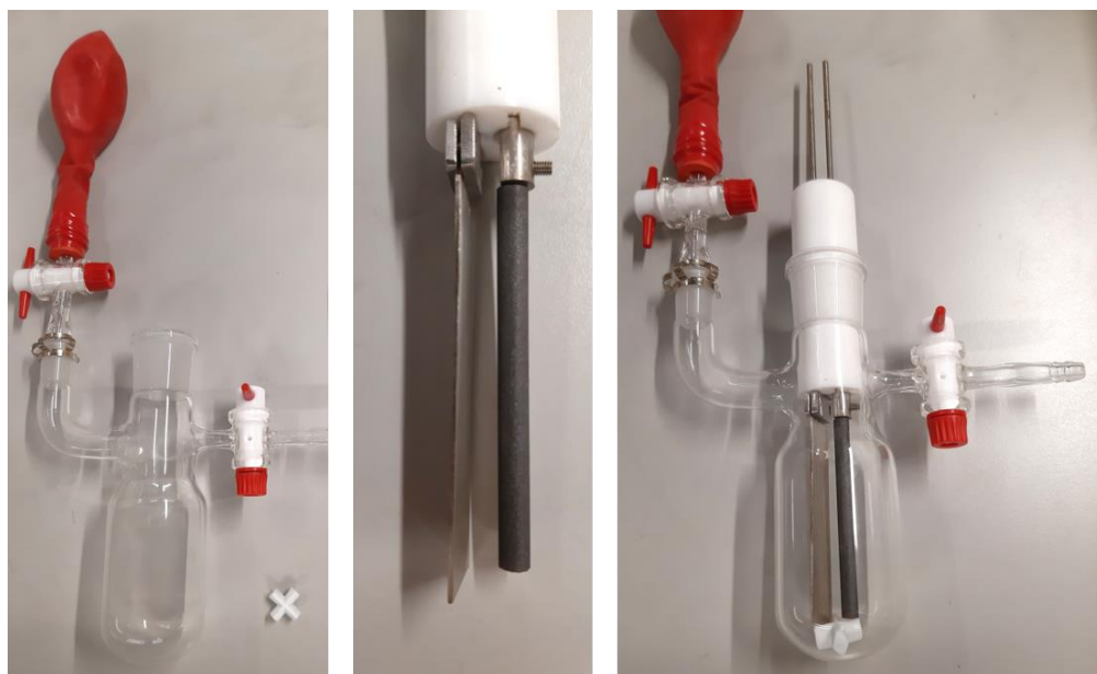
Figure S4: Electrochemical set-up for gram-scale experiment.
