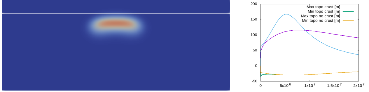
Figure 26: Adding a viscous crust to a model with surface topography. The thermal anomaly spreads horizontally as it collides with the highly viscous crust (left, white solid line). The addition of a crustal layer both dampens and delays the appearance of the topographic maximum and minimum (right).
