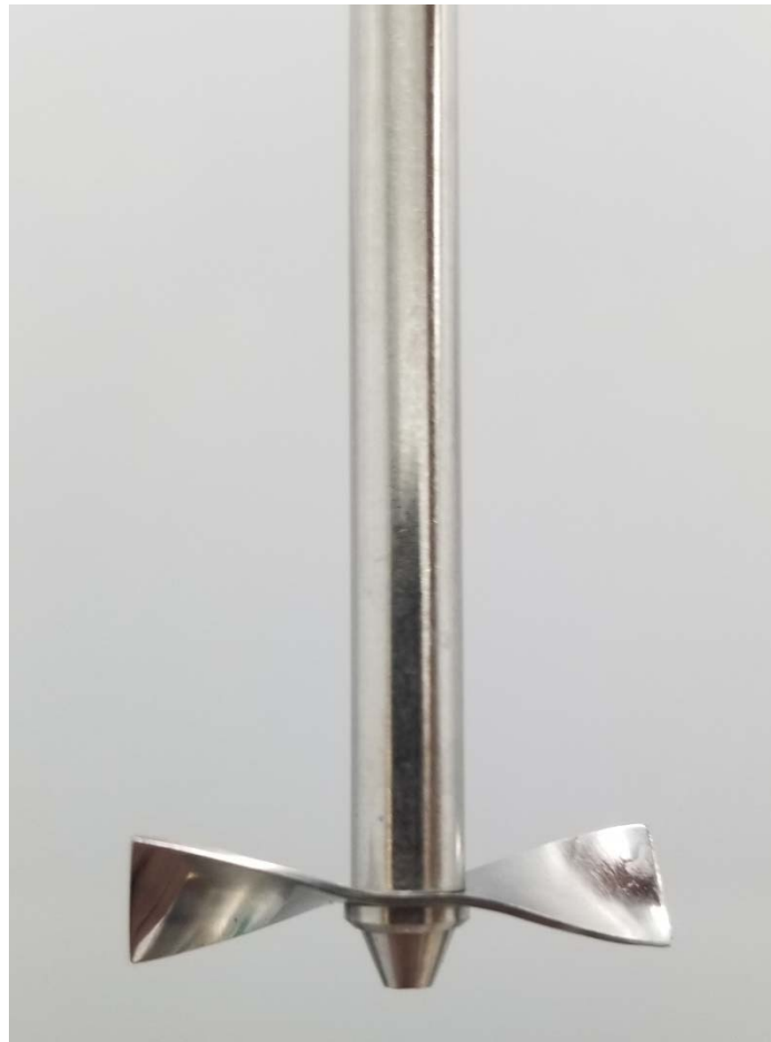
Figure 4-1: Image of the twisted blade used with the FT4 Powder Rheometer (Freeman Technology Ltd., UK).
