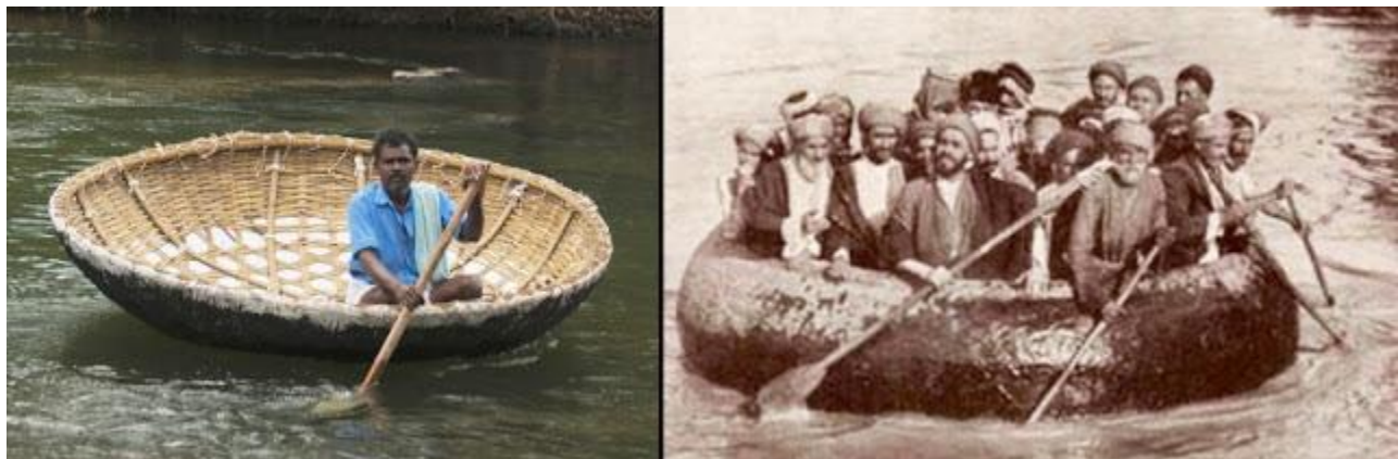
(Left) The basket structure of this boat is visible. (Right) Large basket boats can carry twenty people.
