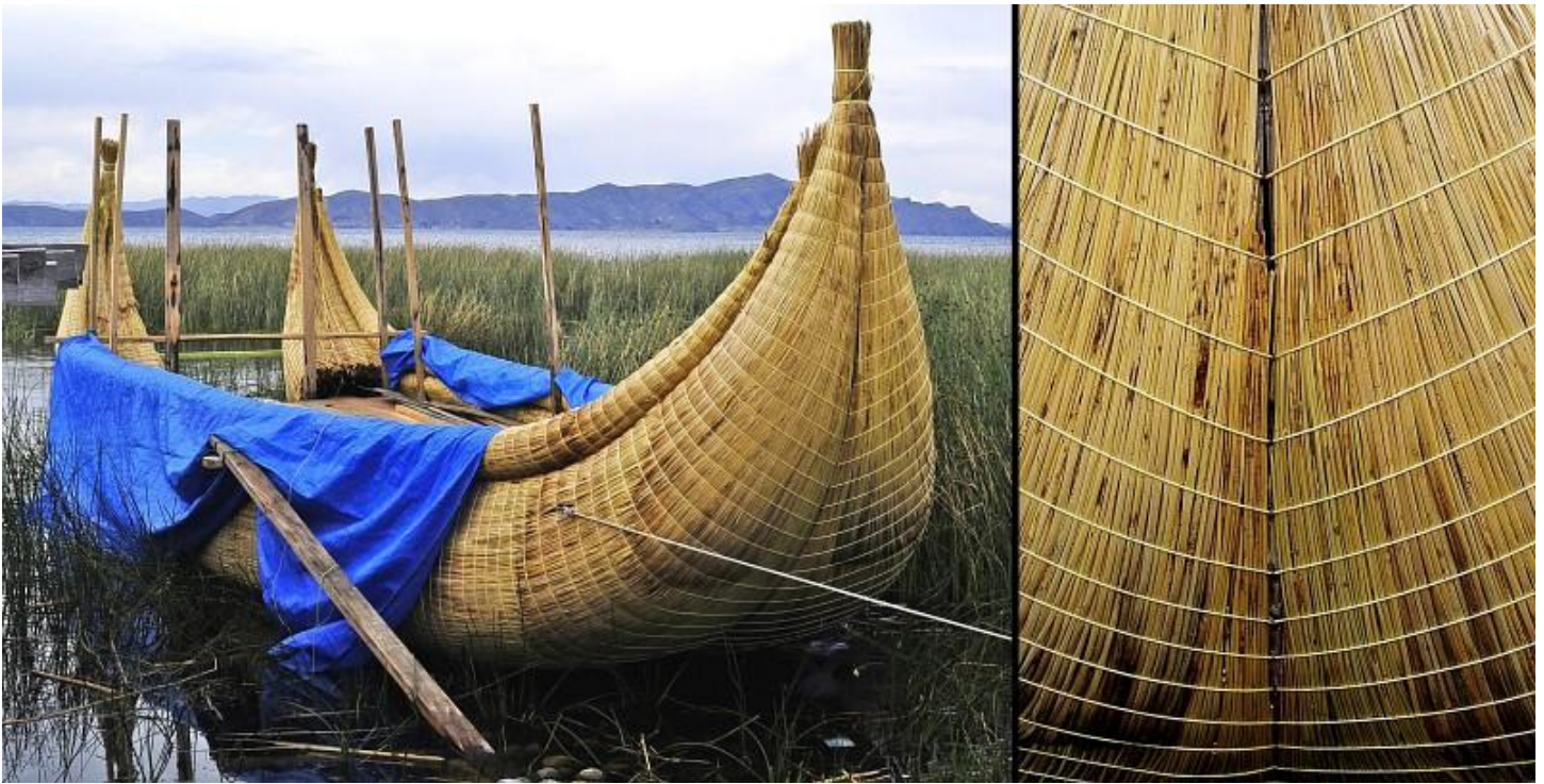
Reed boats in the indigenous pre-Incan community in South America (the Uru or Uros people) made with woven-fiber technology. https://commons.wikimedia.org/wiki/Category:Uros_islands
