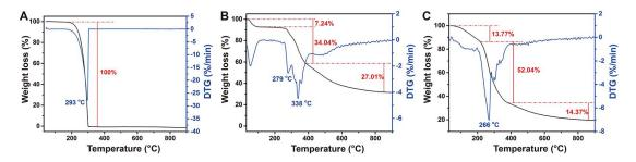
**Figure S1.** TGA profiles and derivative thermogravimetry (DTG) analysis of (A) FLU, (B) PGA nanoparticles, and (C) FLU@PGA nanoparticles.
