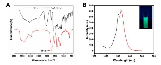
**Figure S6.** (A) FTIR spectra of PGA-FITC nanoparticles. Compared with the spectrum of FITC-cad, the peak at 1727 cm<sup>-1</sup> of PGA-FITC was redshifted to 1716 cm<sup>-1</sup>, and the amino peak at 1673 cm<sup>-1</sup> was weakened, indicating that the PGA-FITC were successfully prepared. (B) Excitation (black) and emission (red) fluorescence spectra of PGA-FITC.
