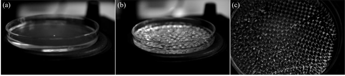
Figure 2.4 : Faraday waves. Vibrating a bath of liquid vertically results in the (a) initially flat surface of the liquid becoming unstable to (b) standing Faraday waves when the driving acceleration amplitude exceeds the Faraday threshold  $\Gamma_F$ . Panels (b) and (c) show the side view and the top view of a typical Faraday wave pattern.
