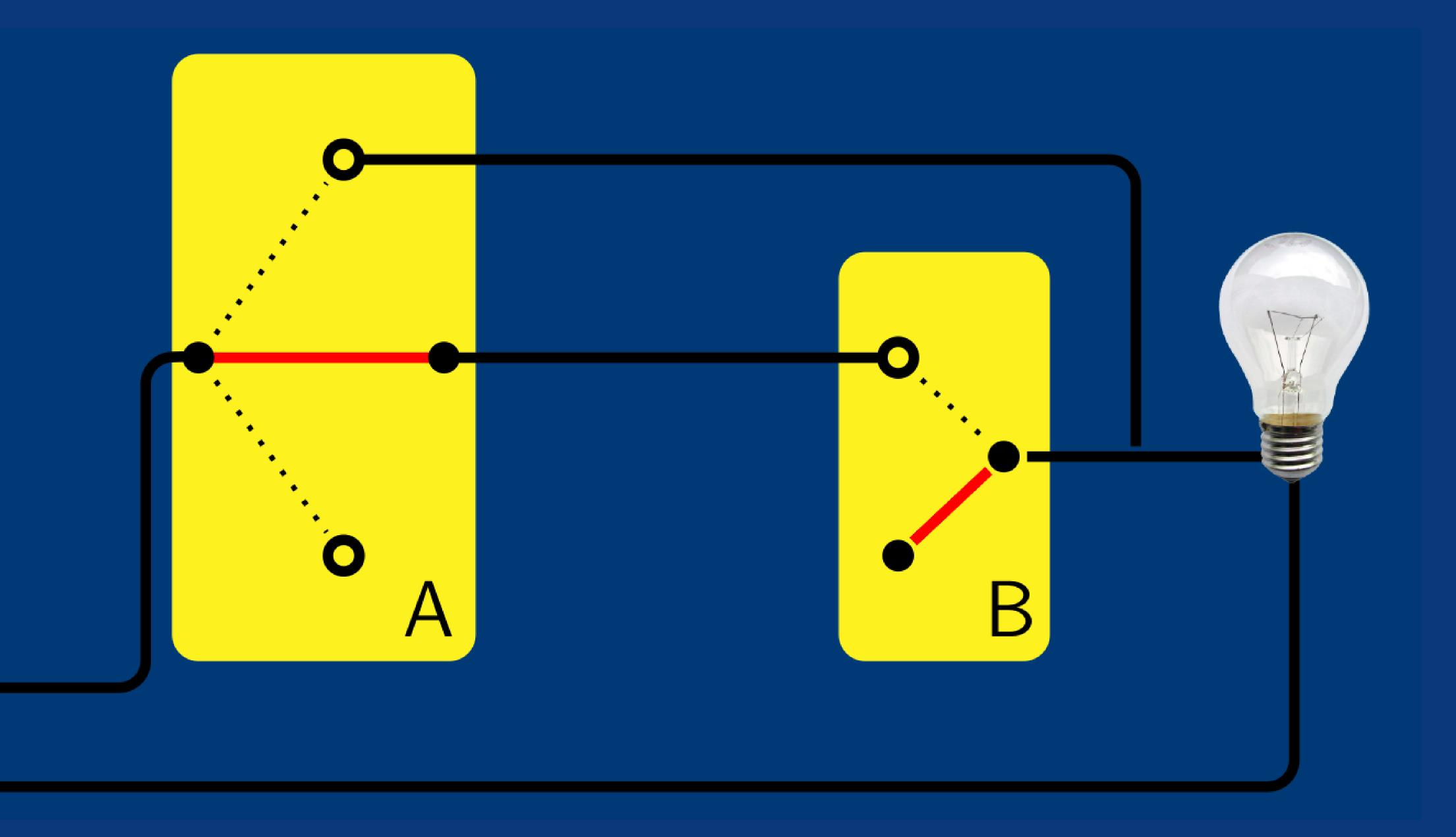
If switch B was up, or switches A and B were up, the light would be on.
