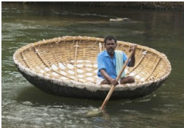
(Left) The basket structure of this boat is visible. (Right) Large basket boats can carry twenty people.
