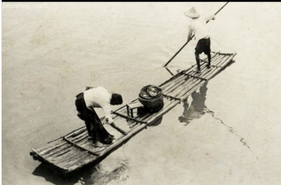
(Top) Children on a raft -- the crossbeams are clearly visible and keep the raft together. (Bottom) A common working bamboo raft in Taiwan. The horizontal right-angled slats are visible.
