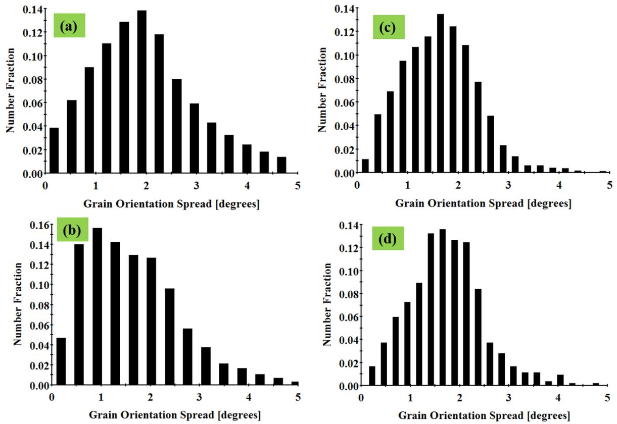
**Figure S5.** Grain orientation spread charts of Cu-Ni alloys in cold rolled state (90% deformation); (a) 100Cu-0Ni, (b) 84.5Cu-15.35Ni, (c) 72.6Cu-27.4Ni and (d) 63Cu-37Ni.
