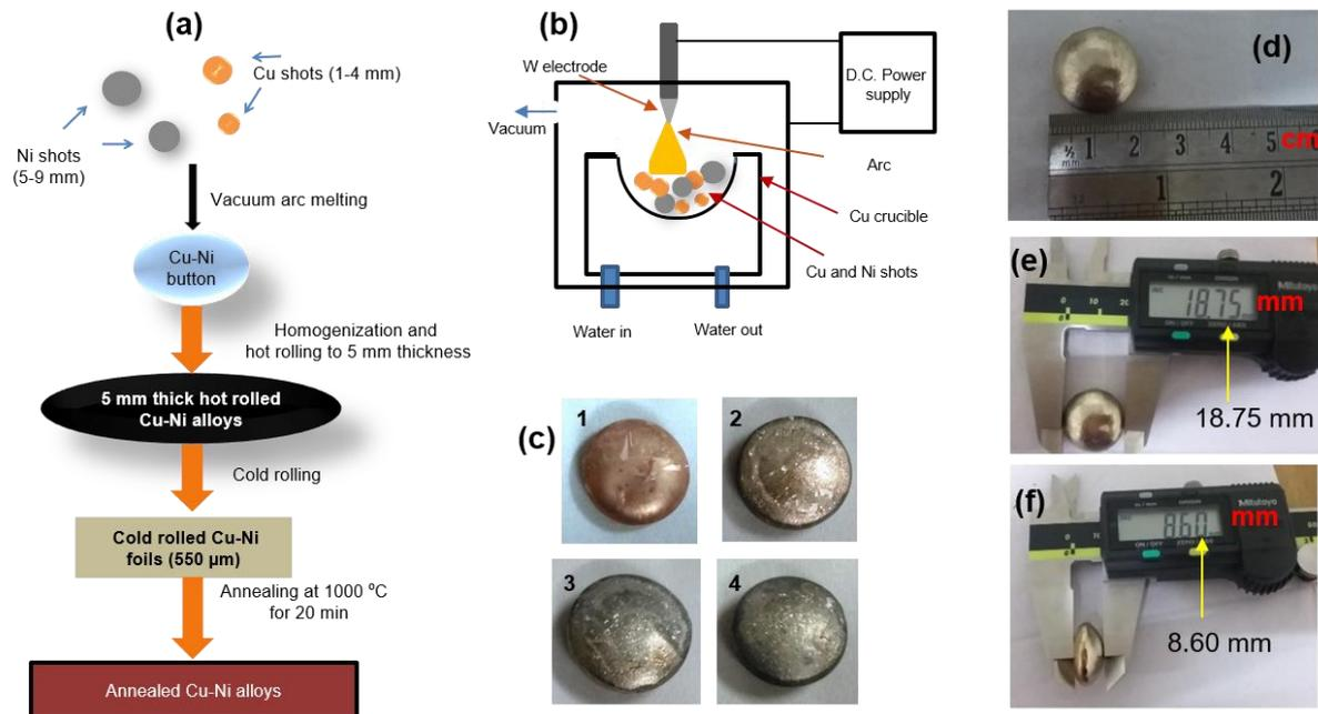
**Figure S1:** (a) Overall schematics of the preparation of Cu-Ni alloy foils. (b) Simplified schematics of vacuum arc melting system. (c) Digital images of prepared Cu-Ni alloy buttons: 1, 2, 3 and 4 corresponds to buttons of compositions 100Cu-0Ni, 84.65Cu-15.35Ni, 72.6Cu-27.4Ni and 63Cu-37Ni, respectively. (d), (e) and (f) show the dimensions of prepared Cu-Ni button.
