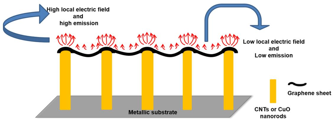
**Figure S7.** Schematic model of field emission from the hybrid structures prepared by transfer of graphene on CNTs or CuO nanorods.
