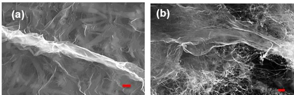
**Figure S6.** FESEM images of graphene transferred from  $^{63}\text{Cu}$ - $^{37}\text{Ni}$  alloy on (a) CuO nanorods and (b) CNTs. Scale bar in both images is 400 nm.
