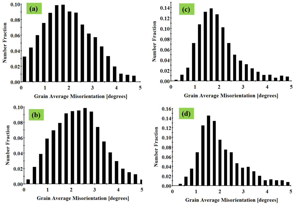
**Figure S4.** Grain average misorientation charts of Cu-Ni alloys in cold rolled state (90% deformation); (a) 100Cu-0Ni, (b) 84.5Cu-15.35Ni, (c) 72.6Cu-27.4Ni and (d) 63Cu-37Ni.
