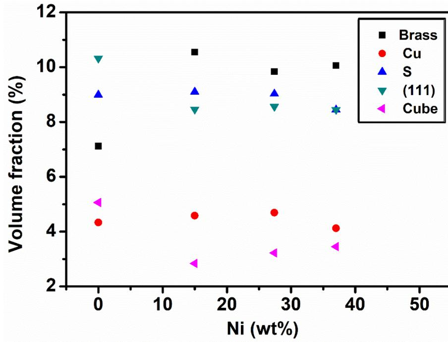
**Figure S3.** Effect of Ni content on volume fraction of different texture components for hot rolled samples.
