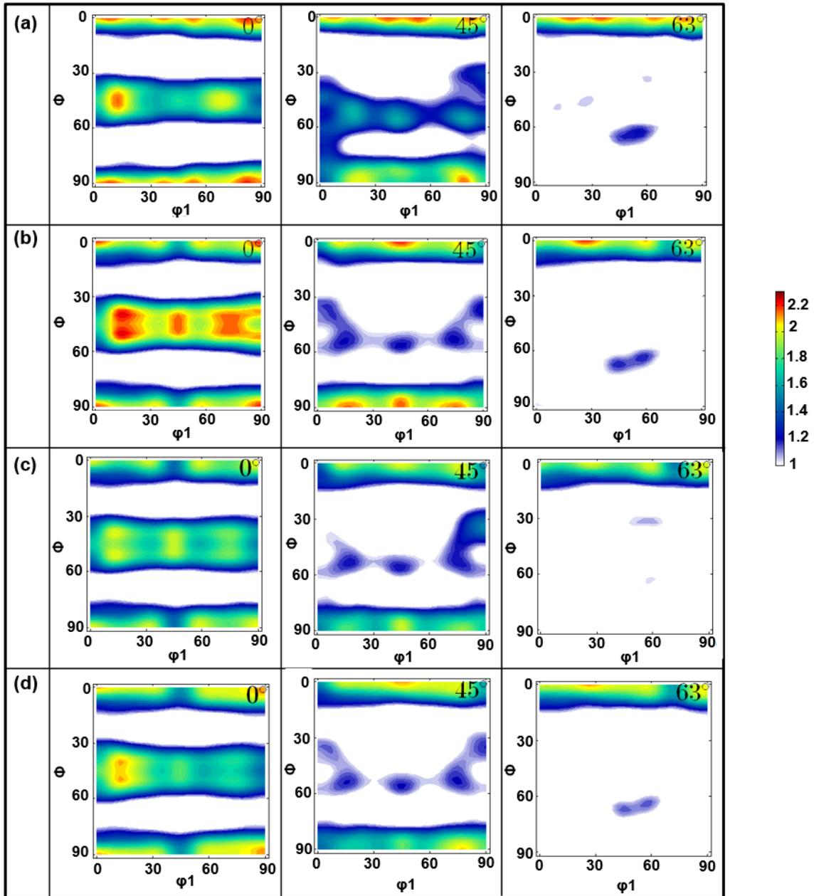
**Figure S2.**  $\phi_2 = 0^\circ$ ,  $45^\circ$  and  $63^\circ$  sections of the ODFs for the Cu-Ni alloys in hot rolled state: (a) 100Cu-0Ni, (b) 84.65Cu-15.35Ni, (c) 72.6Cu-27.4Ni and (d) 63Cu-37Ni (measured by XRD).
