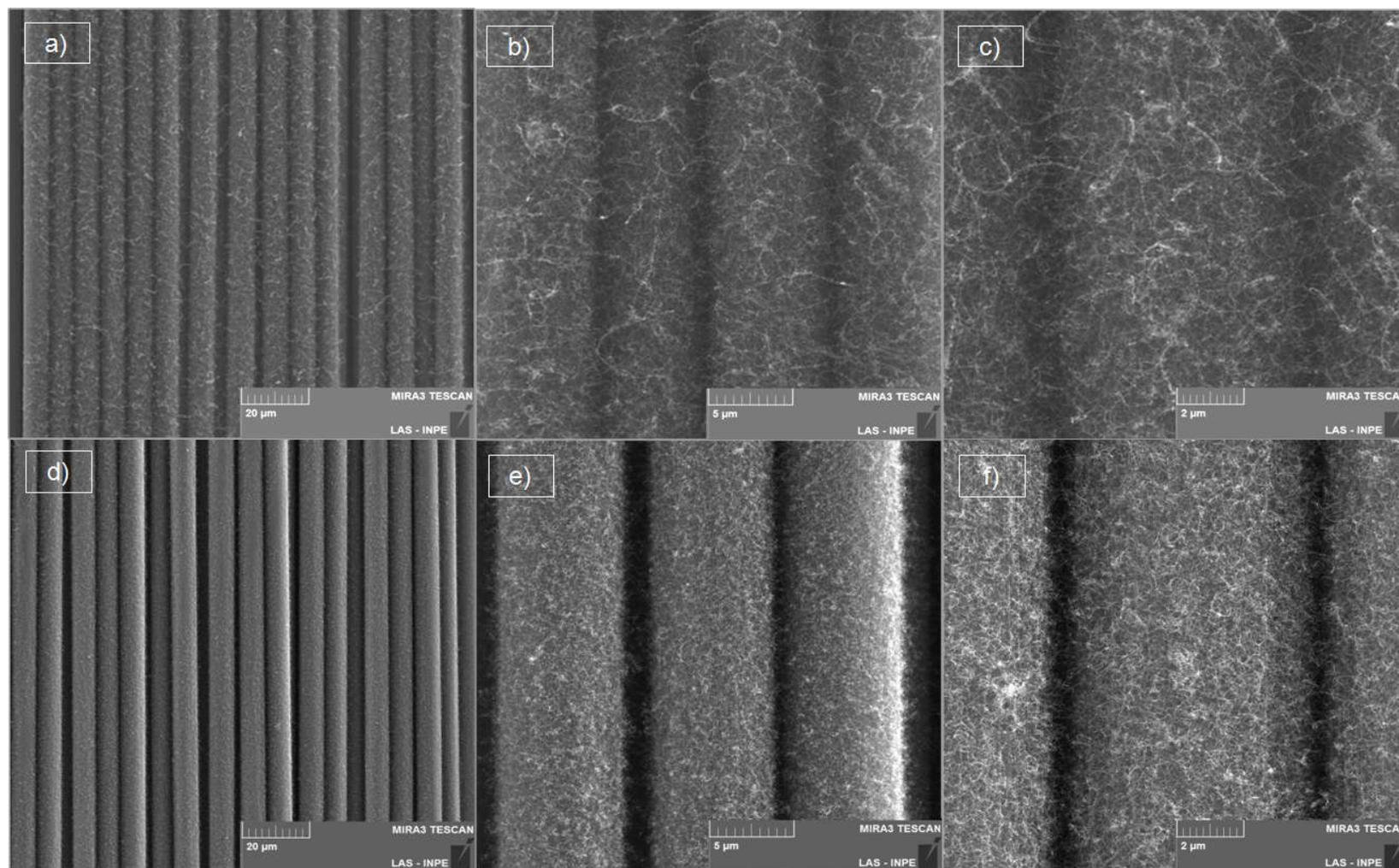
a), b) and c) are different magnifications of CF-OX-H-CNT
