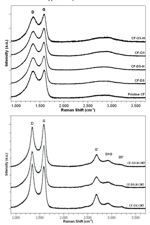
Top: Raman spectra of carbon fiber after the indicated pretreatments
