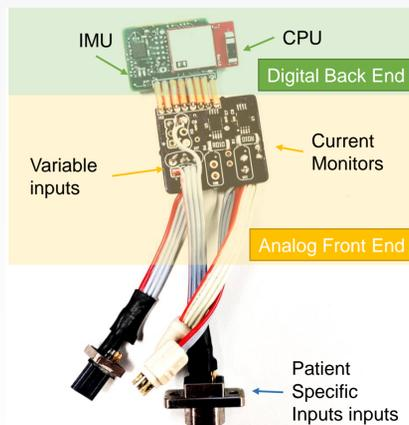
Figure 2 – The MyoLogger module
