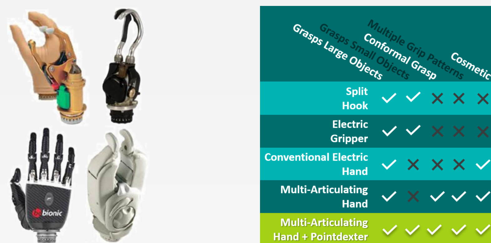
Figure 1 – Commercially available TDs (left) and a feature comparison matrix (right)
