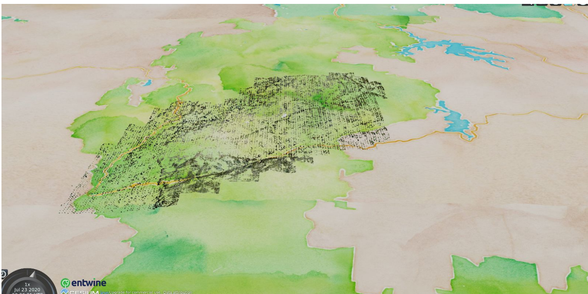
Lidar point cloud over terrain in a CesiumJS web-based virtual globe. Note terrain interference.
