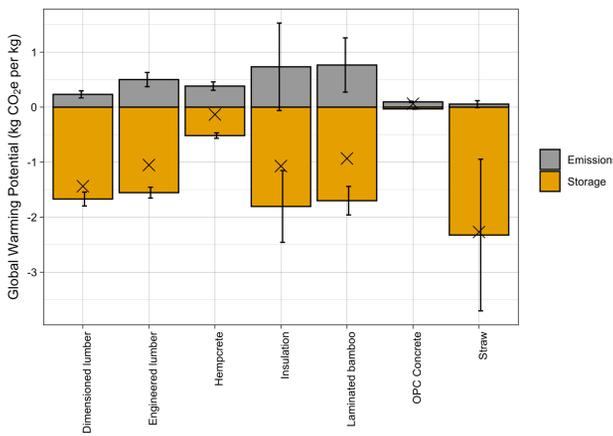
**Figure 1.** Carbon emissions (in gray) compared to carbon storage potential (yellow) of various construction materials. Error bars represent the standard deviations for the data collected, while crosses (X) represent the net cradle-to-gate emissions when carbon storage is considered (for the mean values). Cradle-to-gate emissions are shown for a declared unit of 1kg.
