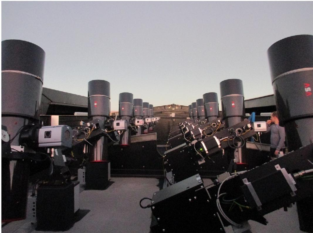
Figure 6.1: The two arrays of 20 cm telescopes used at the NGTS facility (Wheatley et al., 2014).
