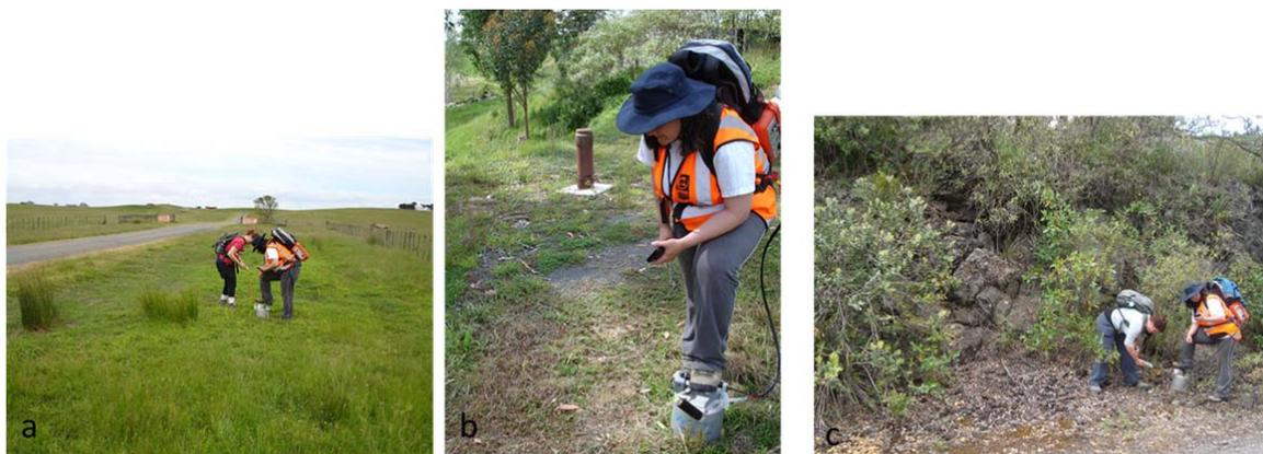
**Figure 8. Measuring soil gas CO<sub>2</sub> flux measurements in a) Puhunui Reserve (5), b) next to a warm water well in Whitford (6), and c) on Rangitoto Volcano (7). These sites represented rural, fault areas in the study. Soil gas concentrations were not measured at these sites due to time and pedology constraints.**
