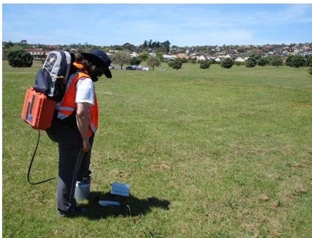
**Figure 7. Measuring soil gas CO<sub>2</sub> fluxes in Lloyd Elsmore Park, Auckland, an urban area overlying a suspected fault, a possible fracture connecting warm water to the surface, and a potential volcanic lineament. Soil gas concentrations were not measured at this site.**
