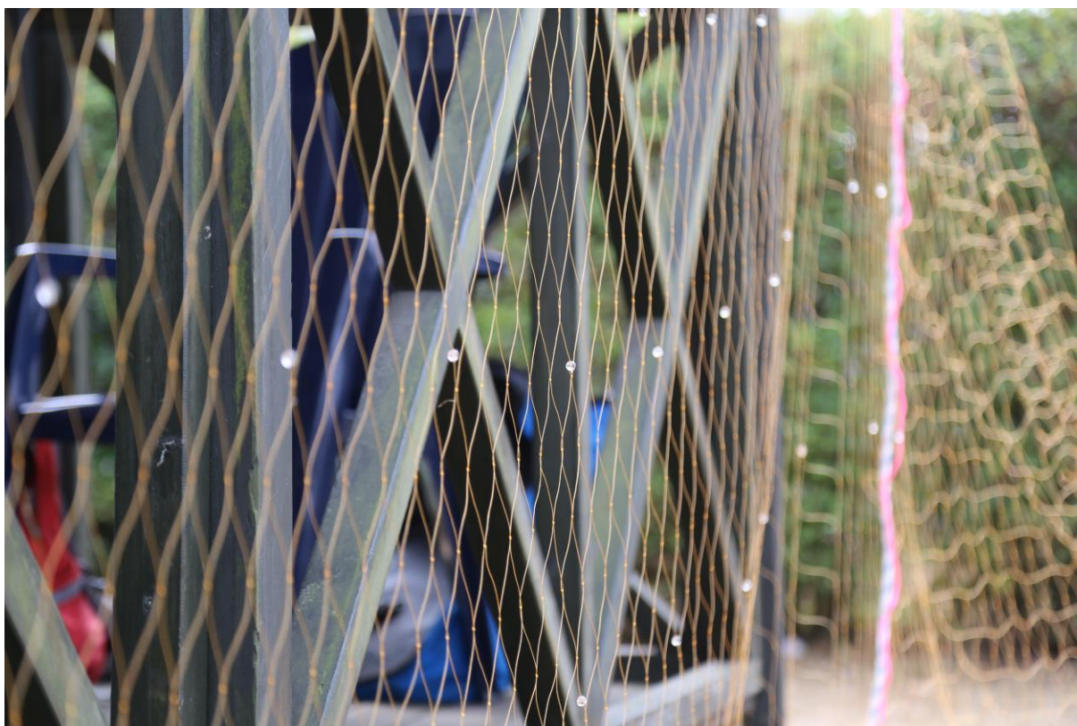
Supplementary Figure 6: standard gillnet with acrylic glass spheres attached at a 30 cm sphere-sphere distance. Photograph taken from angle to render transparent spheres apparent
