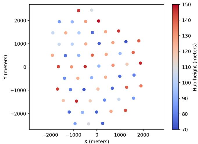
**Figure 5** Wind turbine locations in the Amalia wind farm with associated values for hub-heights that produced the max AEP.
