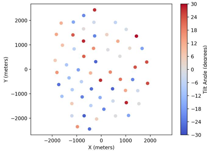
**Figure 6** Wind turbine locations within the boundaries of the Amalia Wind Farm with the optimal tilt angles from test case 1.
