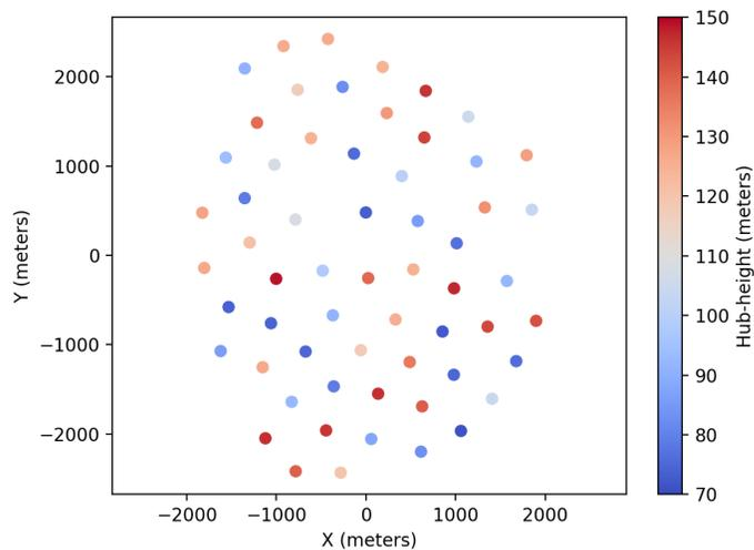
**Figure 7** Wind turbine locations within the boundaries of the Amalia Wind Farm with the optimal hub-heights from test case 2.
