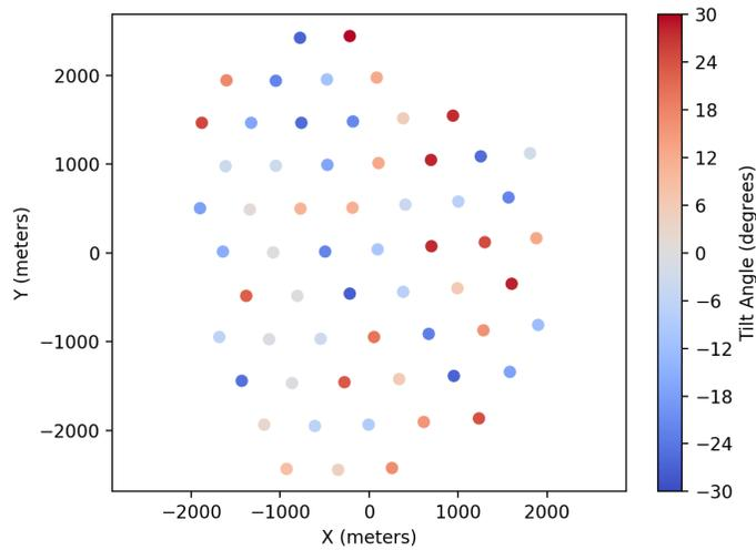
**Figure 4** Wind turbine locations in the Amalia wind farm with associated values for tilt angles that produced the max AEP.
