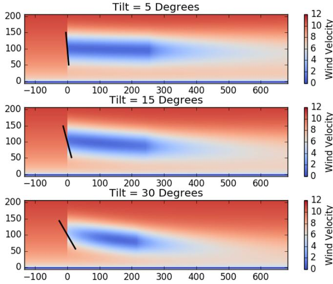
**Figure 1** Visualization of the wake of a single turbine being tilted  $5^\circ$ ,  $15^\circ$ , and  $30^\circ$  using the analytic Gaussian wake model.
