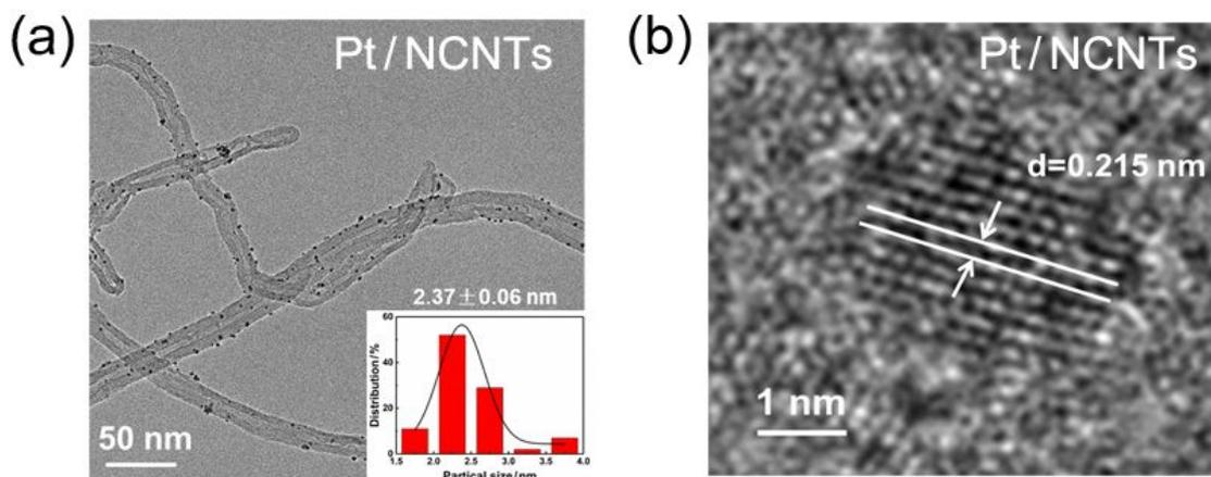
**Figure S5.** (a) TEM image of Pt/NCNTs (insert: Pt particles size distribution). (b) The lattice fringe of Pt in Pt/NCNTs.
