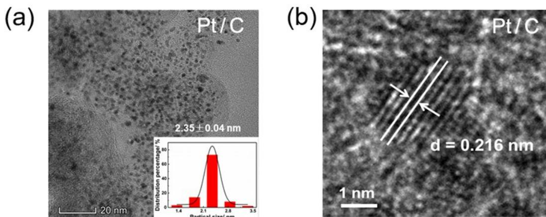
**Figure S4.** (a) TEM image of the commercial Pt/C (JM, 40 wt%) (insert: Pt particles size distribution). (b) The lattice fringe of Pt in Pt/C.
