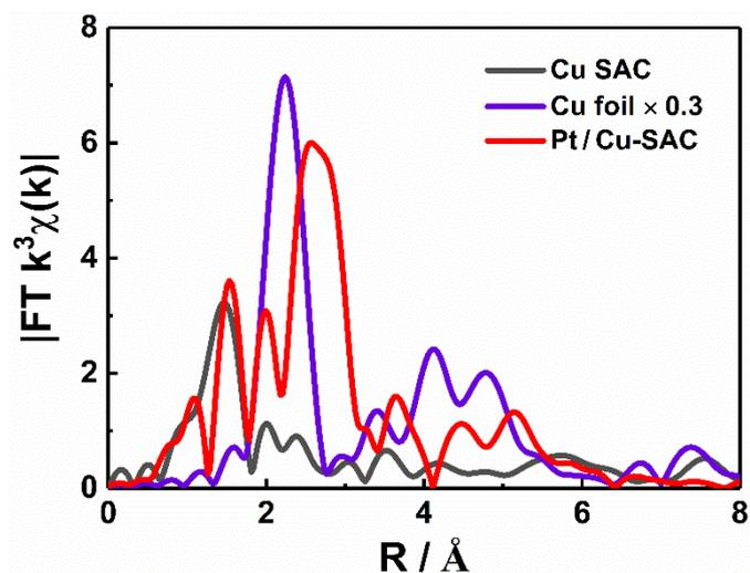
**Figure S3.**  $k^3$ -weighted  $\chi(k)$  function of the extended X-ray absorption fine structure (EXAFS) spectra.
